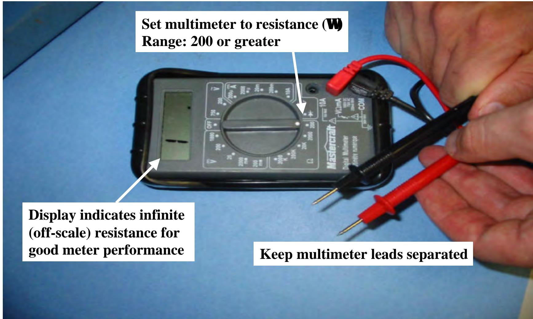
Pic.7 Test multimeter “open” resistance
