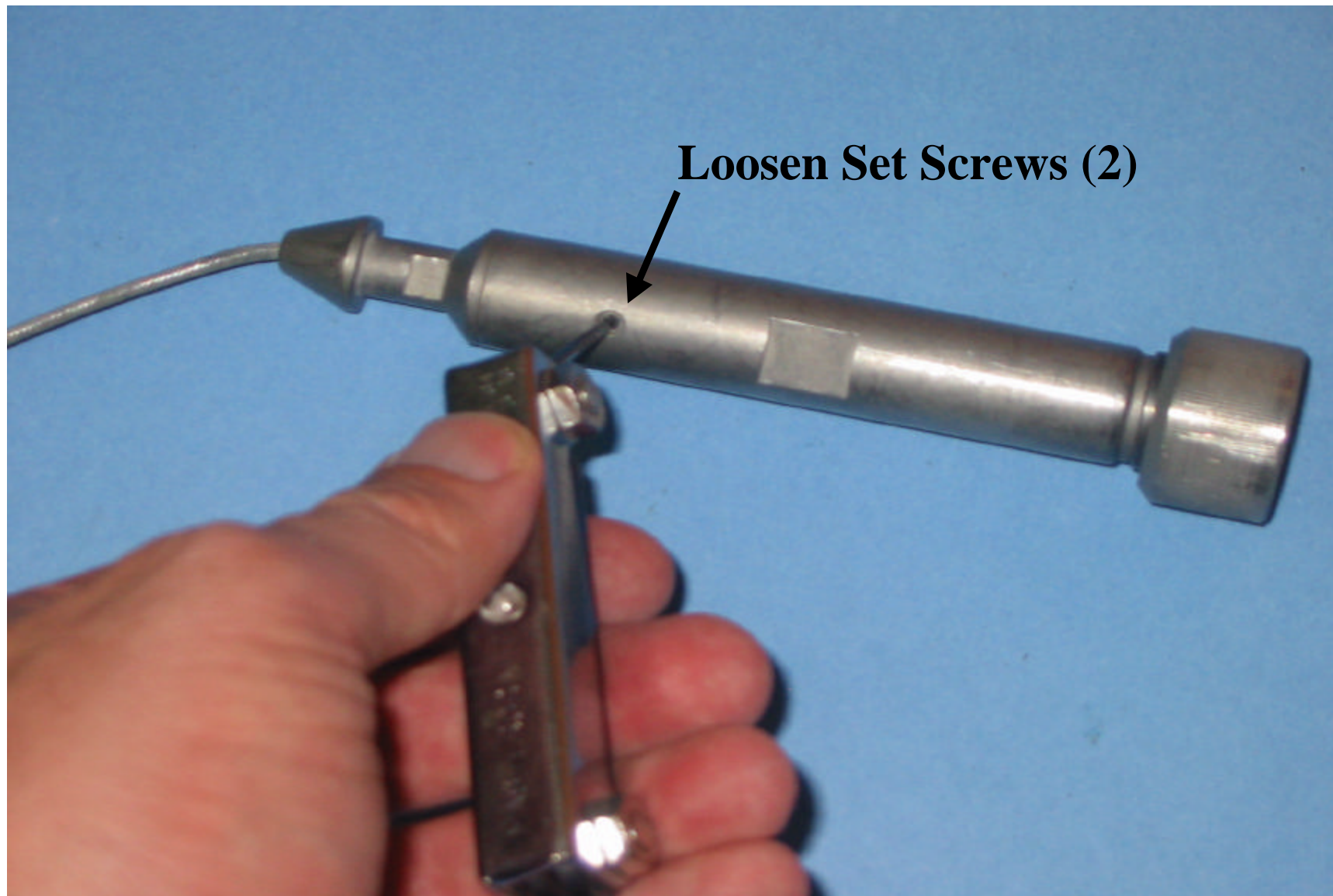
Pic.2 Cablehead Disassembly (1): Loosen set Screws
