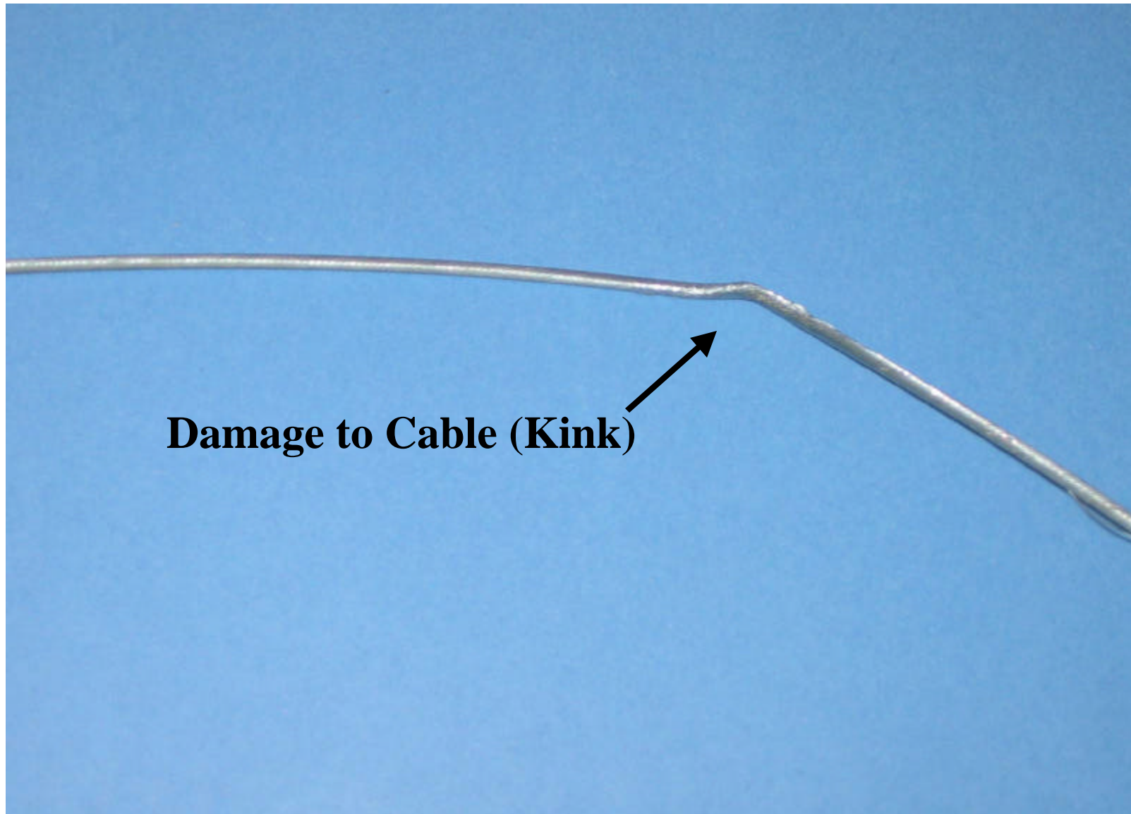
Pic.1 Identification of Cable Damage
