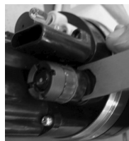
Undo a DO sensor from Sensor Probe
