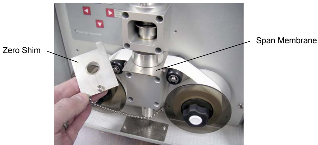
Span Membrane and Zero Shim
