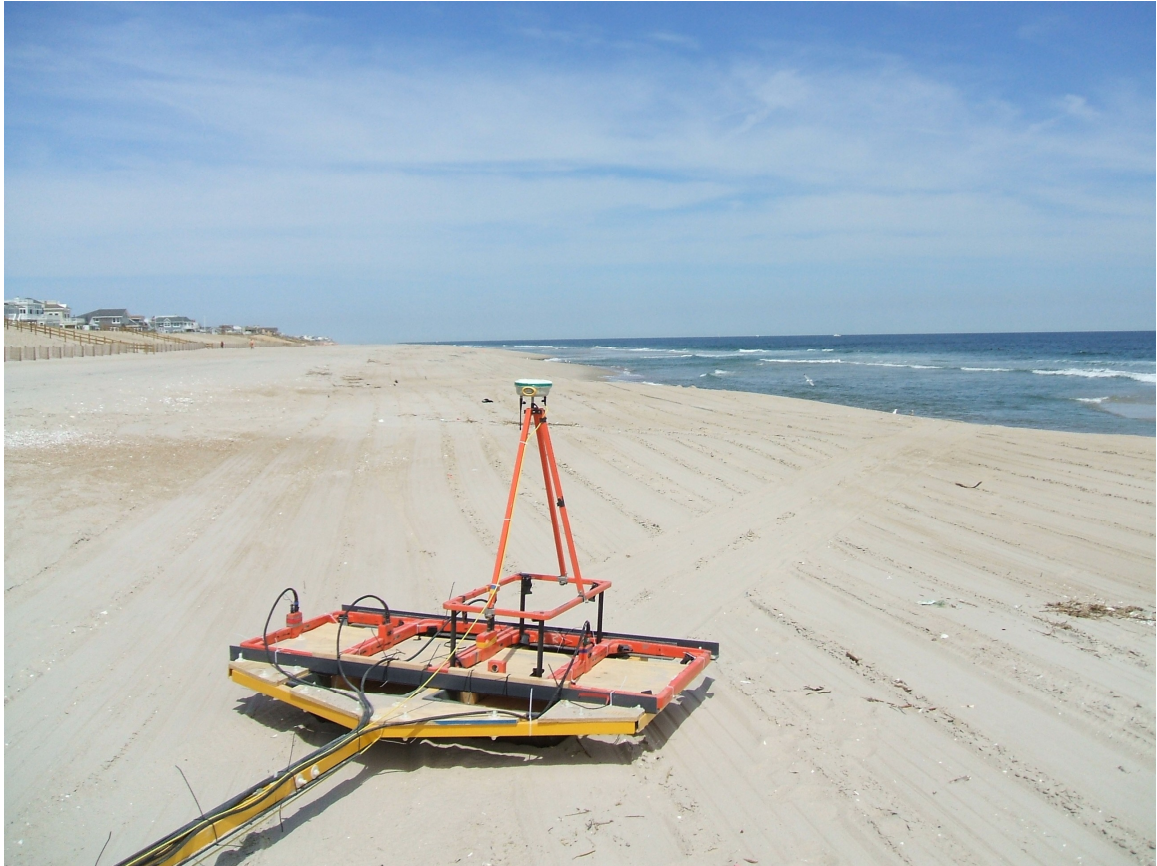
Photo 5-1 Four coil configuration of the EM61-MK2 Towed Array
