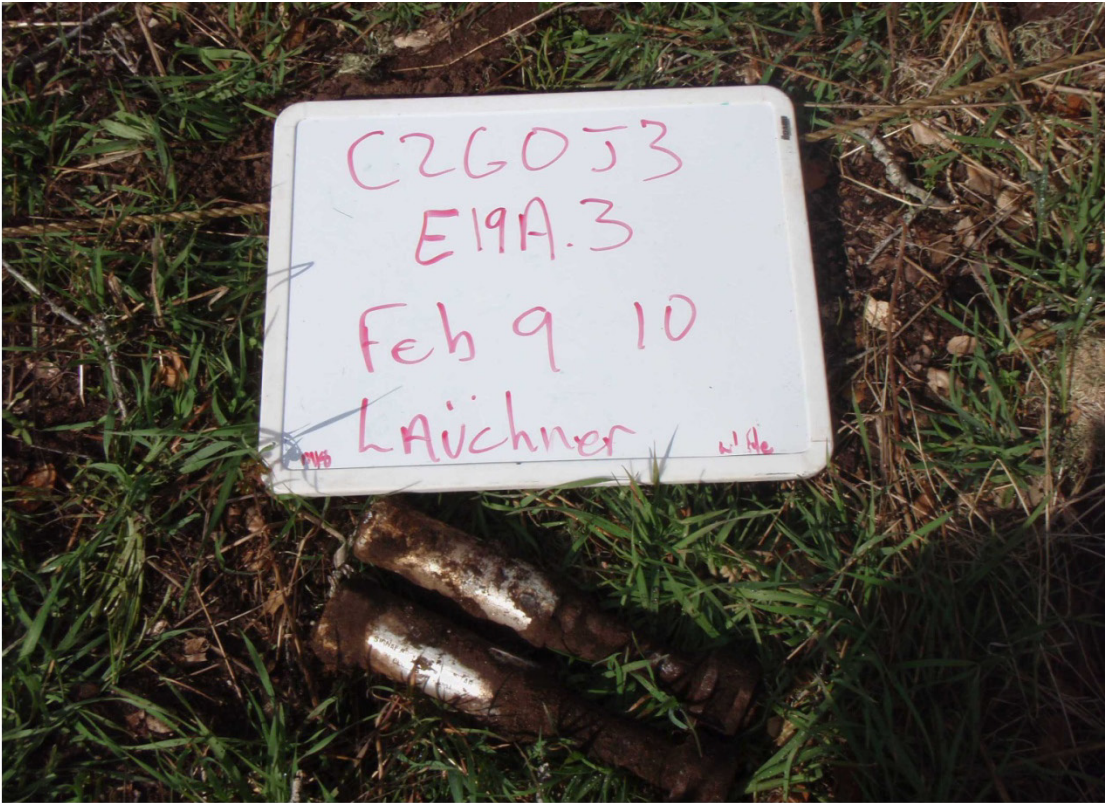
Signal, Ground, Whitestar Cluster, M18A1 (quantity 2) recovered at a depth of 6 inches in Parker Flats Phase II Non-Residential Development Parcel E19.a.3 in grid C2G0J3 on February 9, 2010.
