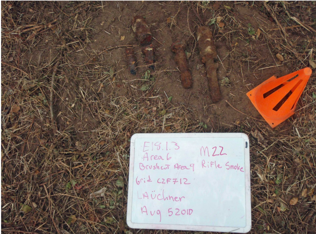
Grenade, Rifle, Smoke, M22 series (quantity 3) recovered at a depth of 6 inches in Parker Flats Phase II Non-Residential Development Parcel E18.1.1 in grid C2F712 on August 5, 2010.
