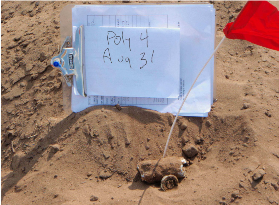
Projectile, 40mm, Parachute, Star, M662 series (quantity 1) recovered at a depth of 0 inches in Parker Flats Phase II Non-Residential Development E19a.3 in grid C2H0A7 on August 31, 2009.
