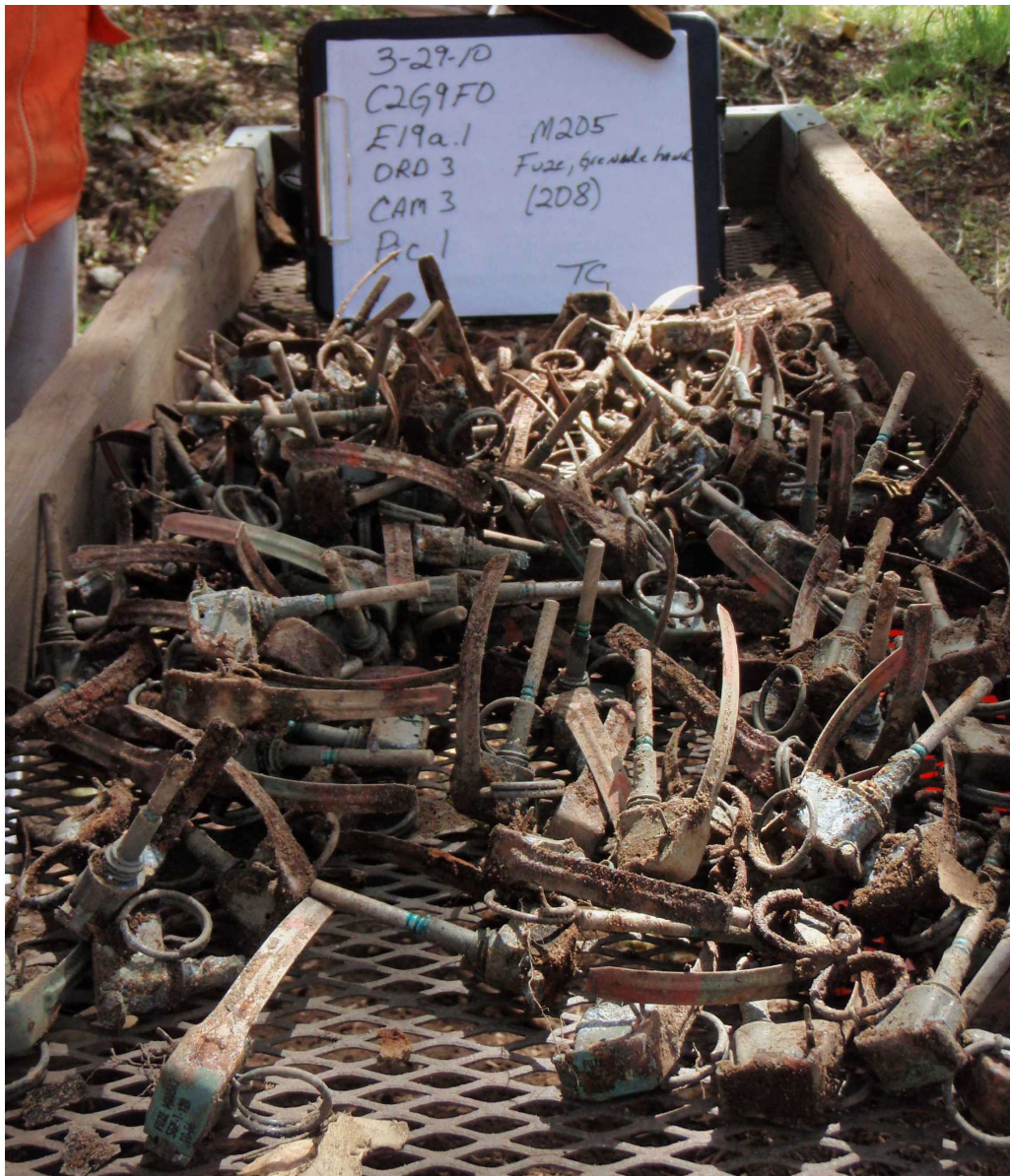
Fuze, Grenade, Hand, Practice, M205 series (quantity 208) recovered at a depth of 12 inches in Parker Flats Phase II Residential Parcel E19a.1 in grid C2G9F0 on March 29, 2010.
