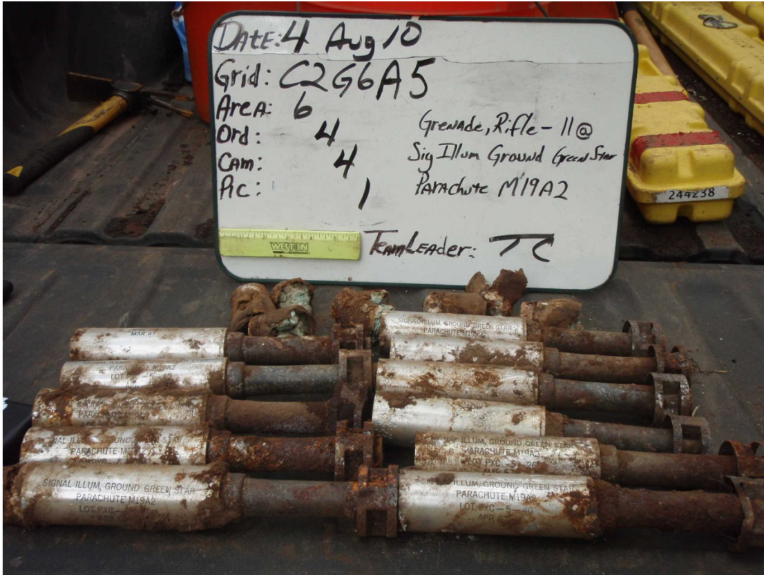
Signal, Illumination, Ground, Rifle, M19A2 series (quantity 11) recovered at a depth of 12 inches in Parker Flats Phase II Residential Parcel E18.1.3 in grid C2G6A5 on August 4, 2010.
