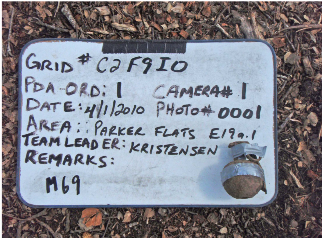
Grenade, Hand, Practice, M69 series (quantity 1) recovered at a depth of 6 inches in Parker Flats Phase II Residential Parcel E19a.1 in grid C2F9I0 on April 1, 2010
