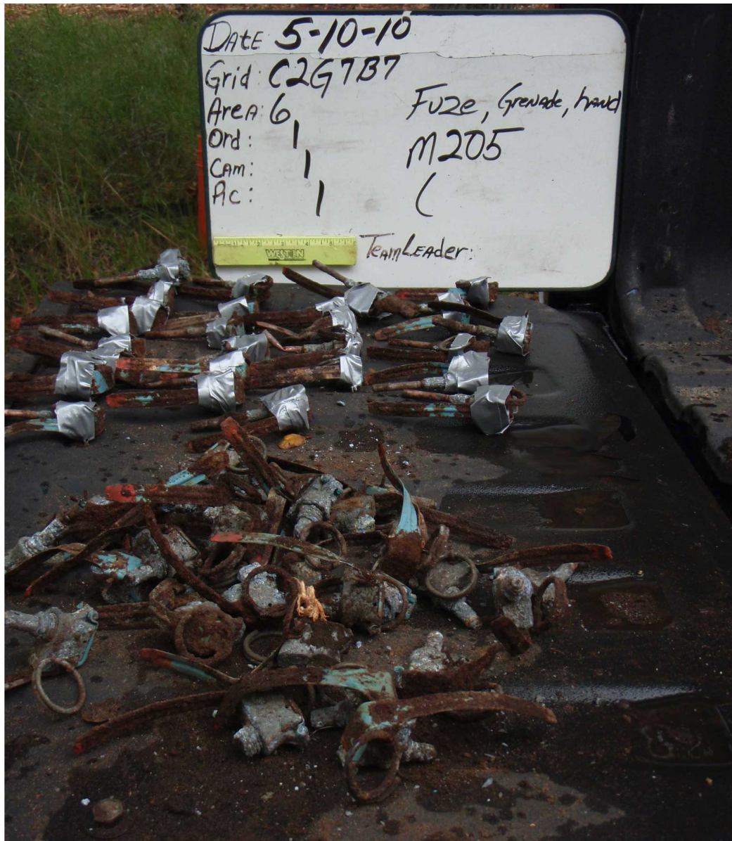
Fuze, Grenade, Hand, M205 series (quantity 56) recovered at a depth of 24 inches in Parker Flats Phase II Residential Parcel E18.1.3 in grid C2G7B7 on May 10, 2010.
