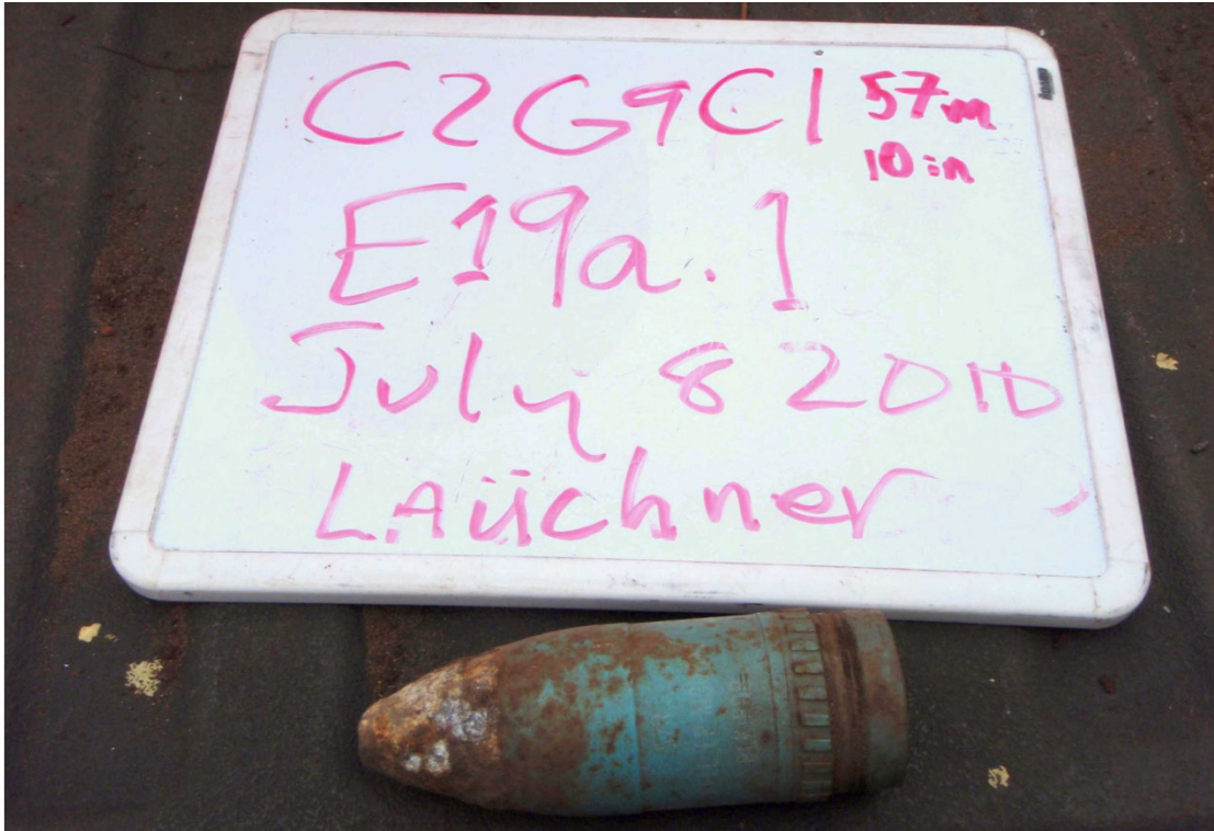
57mm, Projectile, Target Practice, M306 series (quantity 1) recovered at a depth of 10 inches in Parker Flats Phase II Residential Parcel E19.a.1 in grid C2G9C1 on July 8, 2010.
