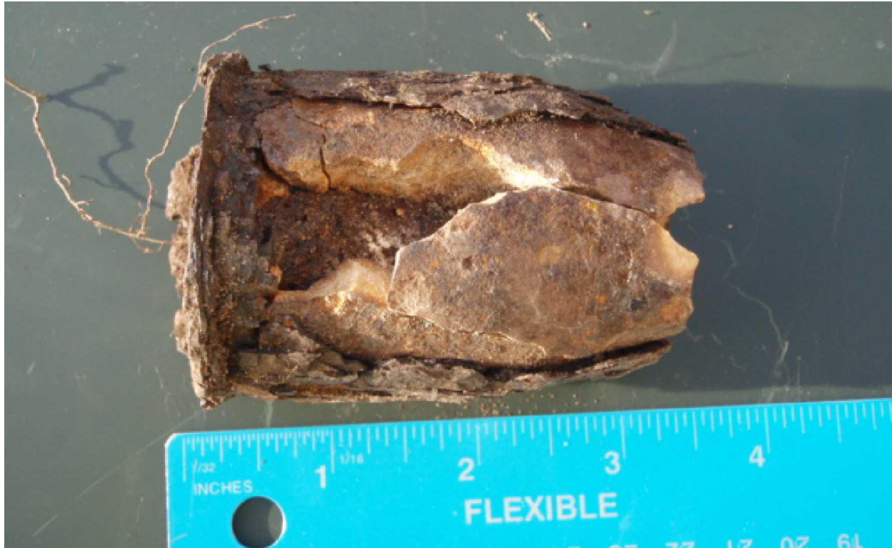
2.36-inch Warhead Nose Cone, HE (quantity 1) recovered at a depth of 6 inches in Parker Flats Phase II Non-Residential Development Parcel E19a.3 grid C3G1B1 on September 21, 2010.
