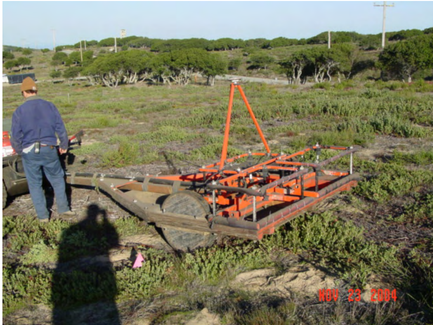
a. Towed-array with three EM-61 MKII sensors.
