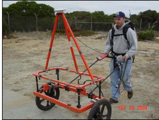
6 7 Photograph 2—Three sets of geophysical data were collected with the EM61-MK2 system pictured.
