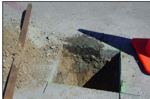
19 20 Photograph 1—Approximately 14-in.-squares were cut into the asphalt so test items could be buried 21 underneath it.
