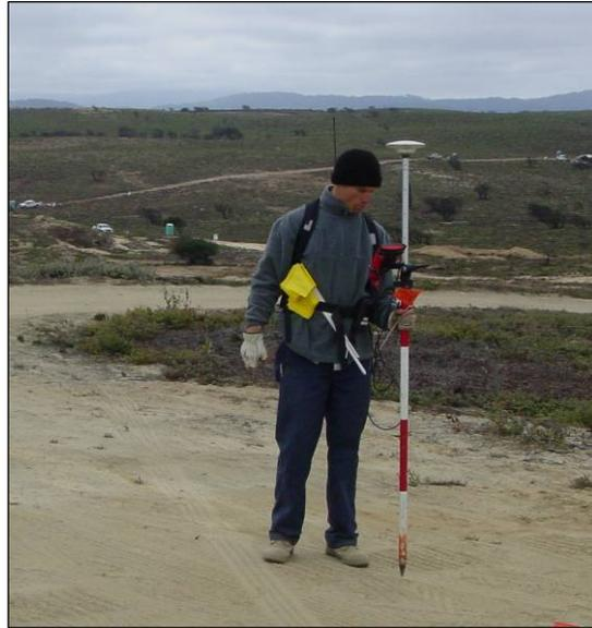
5 *Photograph 6-3 — A Leica GPS receiver attached to the digital survey instruments accurately*
