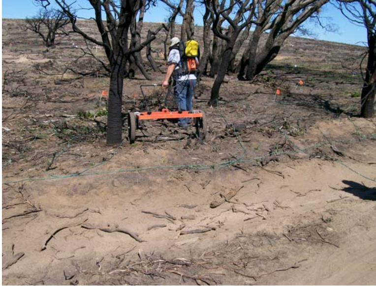
Photograph 21 Single EM61 Unit
