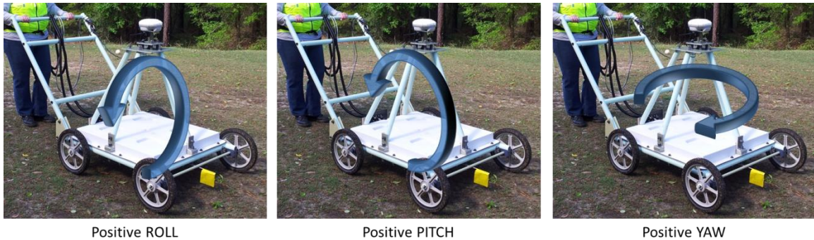
Figure 14. Positive ROLL, PITCH, and YAW rotations of the IMU
