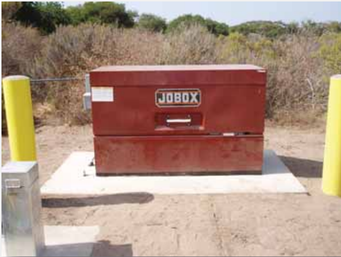
Photo 25. Metal box mounted on well MW-OU1-46-AD.
