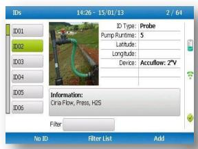
By selecting 'Key 5' the operator can toggle between showing 30 IDs and showing 5 IDs with more detailed information relating to the chosen ID.
