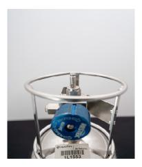
3) Release the sleeve once fully seated. Gently pull up on flow controller to make sure the fittings are properly connected.
