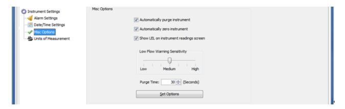
Under the miscellaneous options interface the user can change the following instrument settings:
