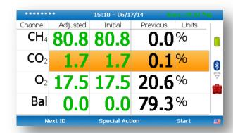
You can use key 4 and key 6 to switch between the gases page and the pressure & flow page. This feature is only available on analyzers running on firmware version 1.11 or later.
