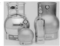
range. When the sample has been collected, the valve is closed and the canister is returned to the laboratory. Canisters range in volume from less than 1 liter (L) to 6 L. In general, 6 L canisters are used to collect ambient air samples and samples requiring time integration greater than 2 hours. One liter canisters are typically used for taking high concentration (i.e., greater than 5 ppbv) samples not requiring time integration such as soil vapor.
