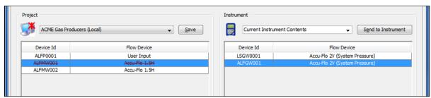
The computer Icon will now display a red asterisk\* over the image . This indicates that the IDs are NOT saved. Deleted IDs are displayed with a line through the information on the screen. To restore a deleted ID, right click on the ID and click **Restore Selected Device ID(s)**.
