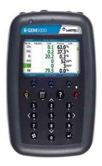
The GEM5000 gas analyzer is designed to monitor landfill gas extraction systems.
