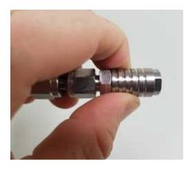
2) Place the female end of the QT fitting over the male QT fitting located on the top of the canister.
