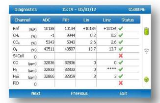
Select soft-key 'Next' to display the next screen, 'Previous' to return to the previous 3) screen, or select soft-key 'Exit' to exit this screen and return to the 'Device Settings' menu.
