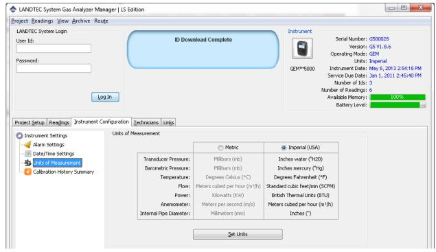
The Units of Measurement interface allows users to select whether to operate the instrument in metric or imperial units. The units for each parameter are displayed on the screen.
