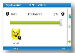
2) Keys 4 and 6 can be used to adjust the brightness of the display screen.
