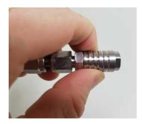
4) Place the female end of the QT valve over the male QT valve located on the top of the canister then release the sleeve once fully seated. Gently pull up on the filter/gauge pair to make sure they are fully connected to the canister.
