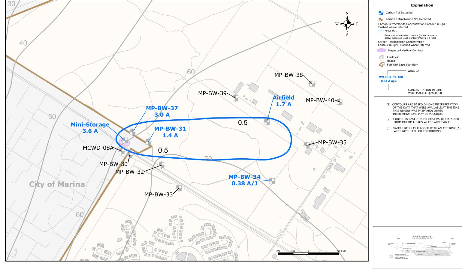
Carbon Tetrachloride Concentration Contour in ug/L;
