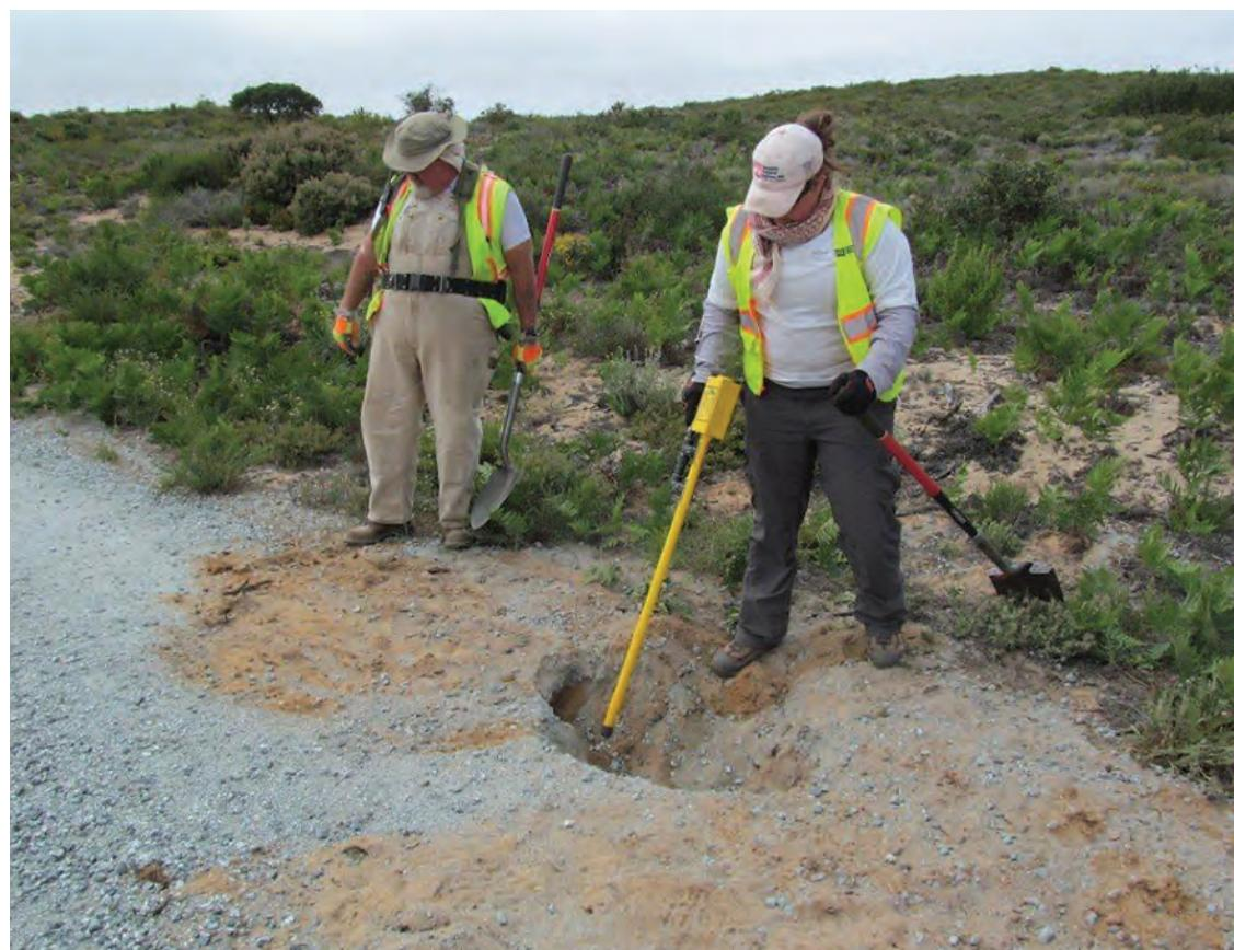
2011 Munitions Clearance Work using a Schonstedt Magnetometer
