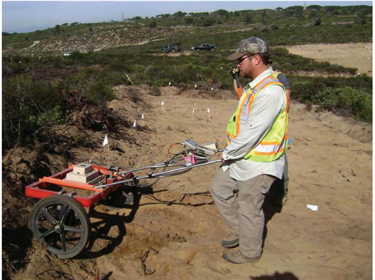
2011 Munitions Clearance Work using an electromagnetic metal detector
