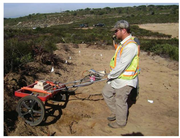
2011 Munitions Clearance Work using an electromagnetic metal detector
