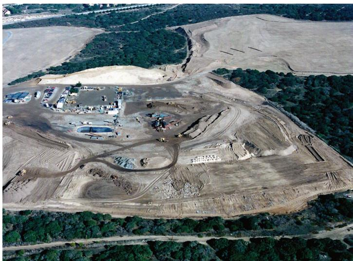
In 1997, landfill cleanup and cover construction began. In 2005 and 2006, a gas extraction system and thermal treatment unit were installed.
