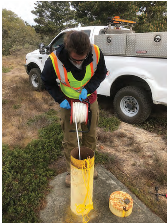
Groundwater monitoring left to right: Equipment setup for multiport well monitoring; measuring water level in a monitoring well; and preparing samples for sending to the laboratory. Photos courtesy of D. Lieberman, AHTNA
