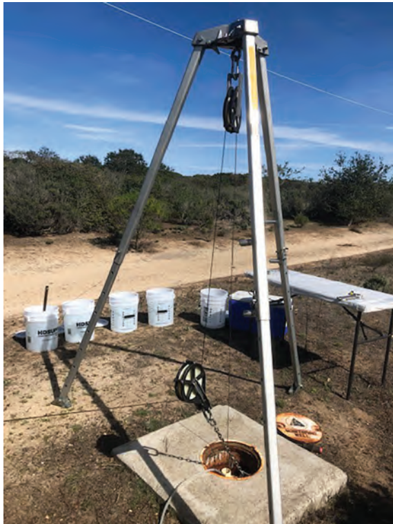
Groundwater monitoring left to right: Equipment setup for multiport well monitoring; measuring water level in a monitoring well; and preparing samples for sending to the laboratory. Photos courtesy of D. Lieberman, AHTNA
