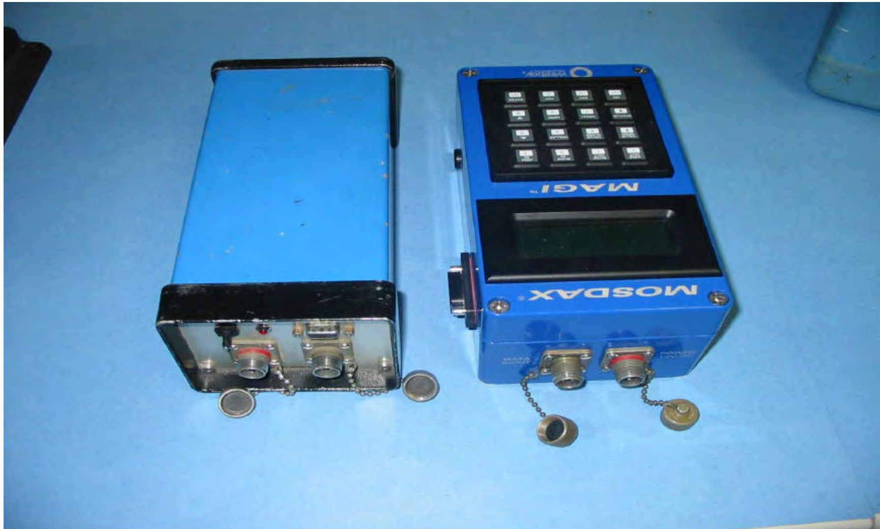
Pic.1 Computer Interface Units, old and new: MPCl model 2522 (left) and MAGI model 2536 (right)
