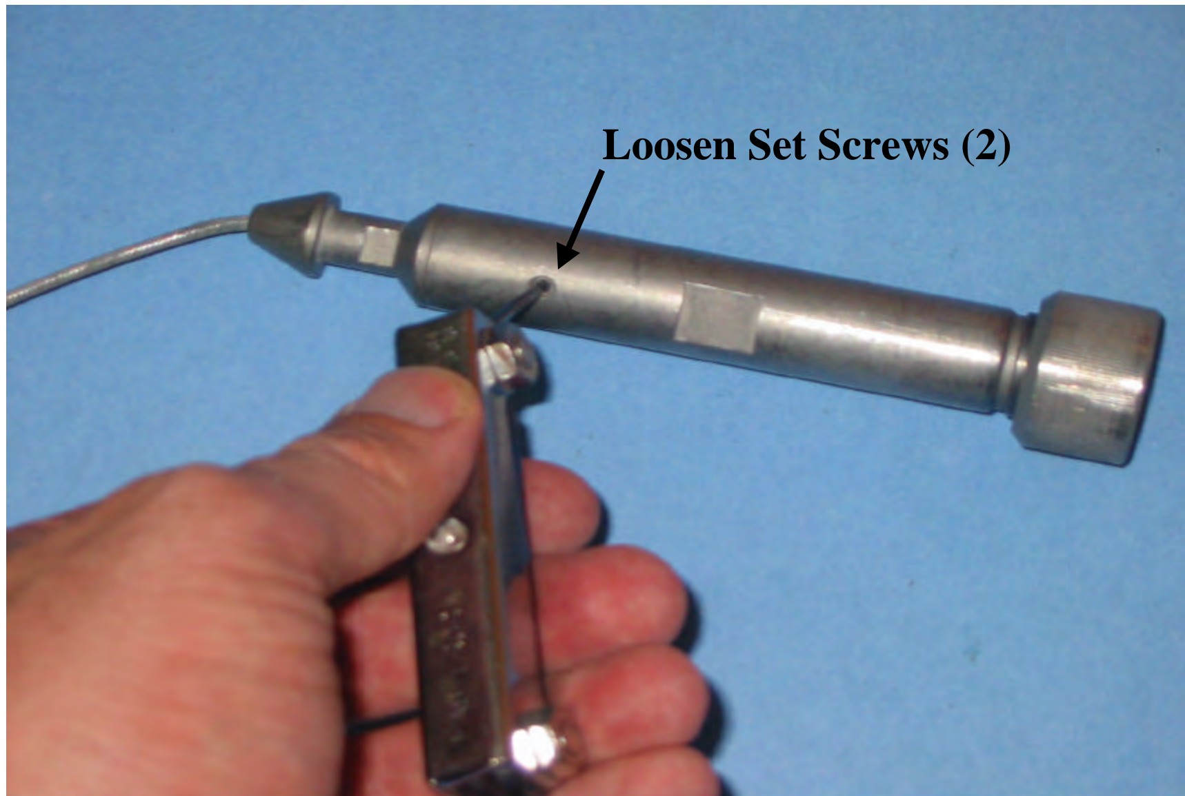
Pic.2 Cablehead Disassembly (1): Loosen set Screws
