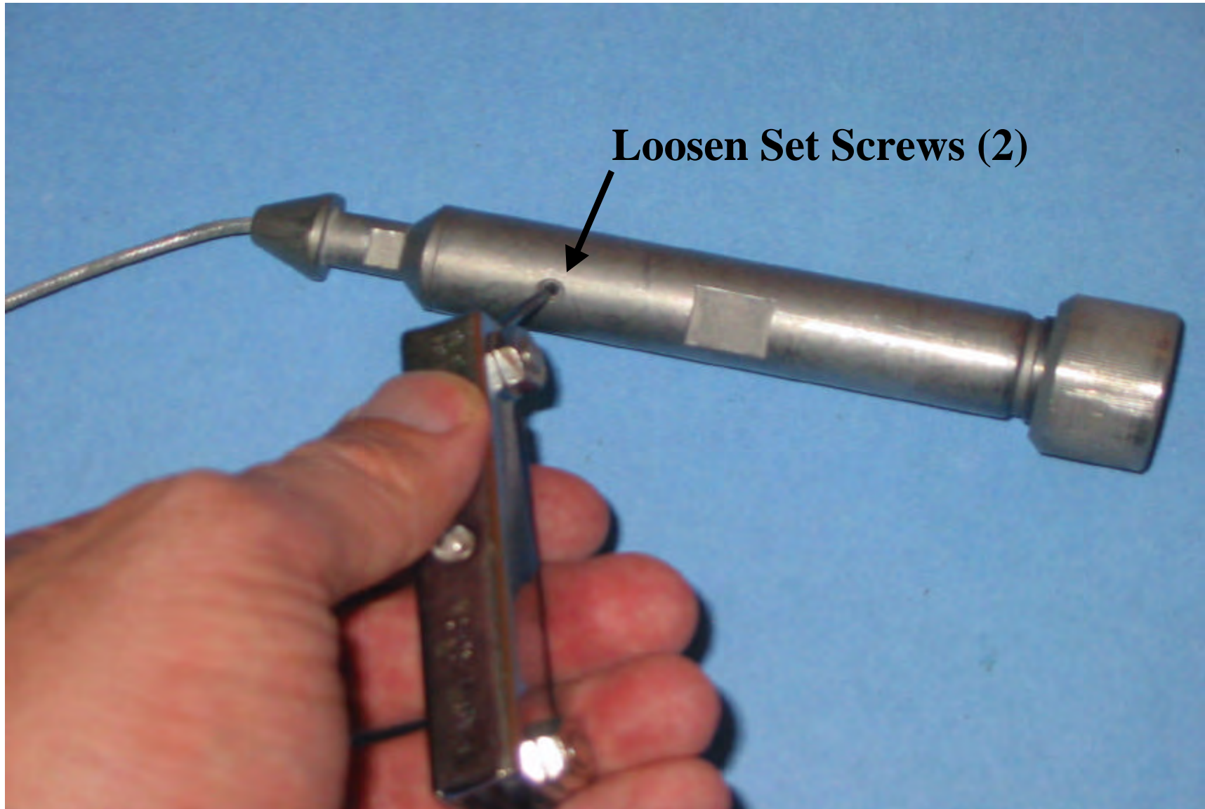
Pic.2 Cablehead Disassembly (1): Loosen set Screws
