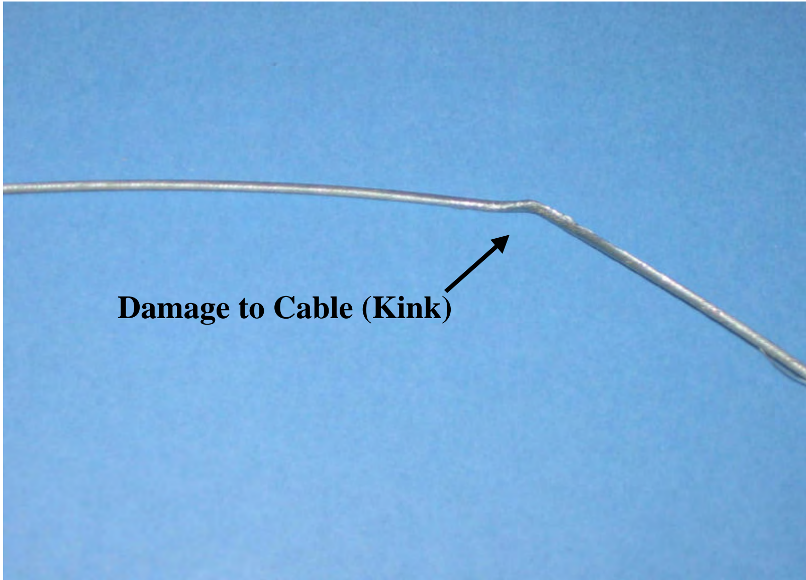
Pic.1 Identification of Cable Damage
