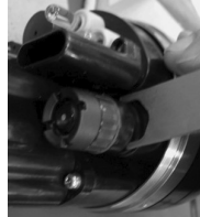
Undo a DO sensor from Sensor Probe
