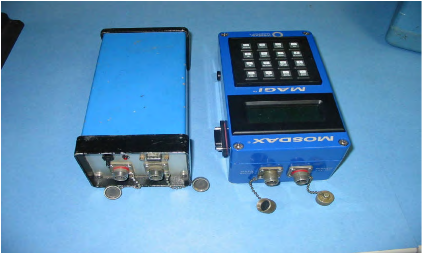
Pic.1 Computer Interface Units, old and new: MPCI model 2522 (left) and MAGI model 2536 (right)
