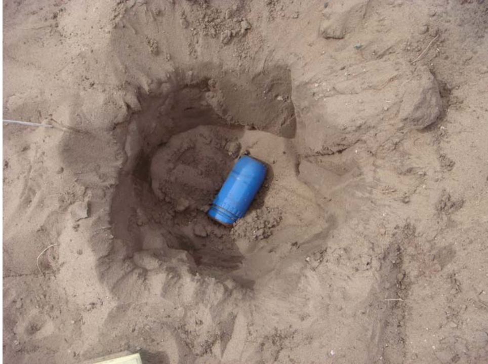
Test Plot 2 - Seed Item 3, 57 mm, buried depth = 6 inches
