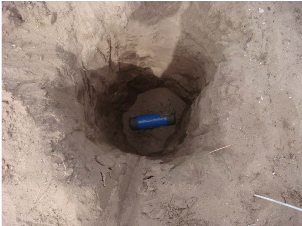
Test Plot 2 - Seed Item 8, 37 mm (pipe), buried depth = 18 inches
