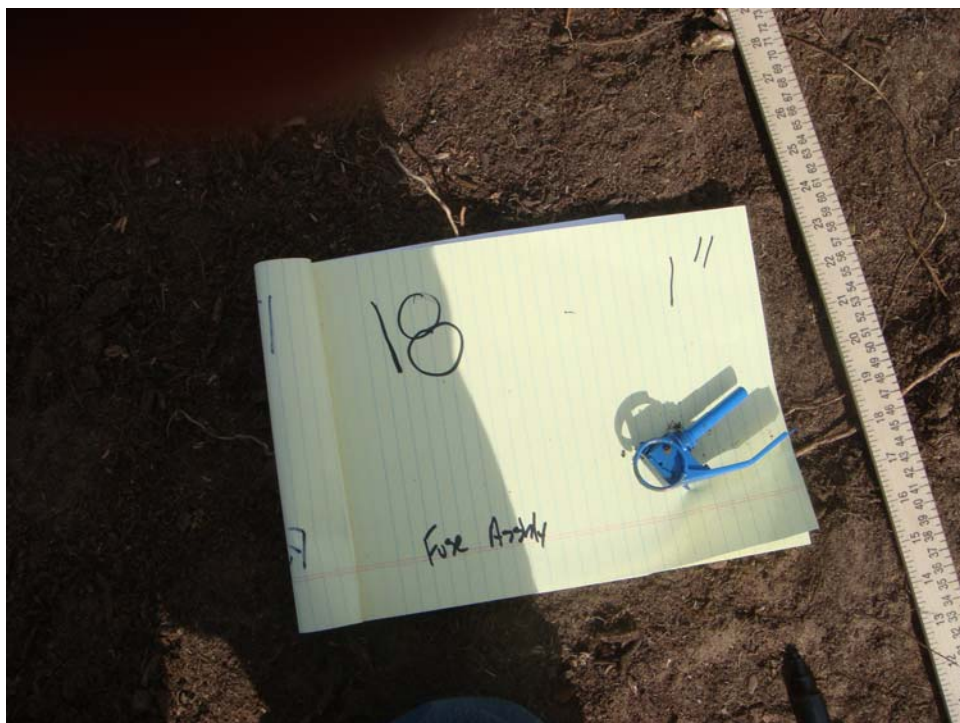
Test Plot 1 - Seed Item 18, Grenade Fuze Assembly, buried depth = 1 inch
