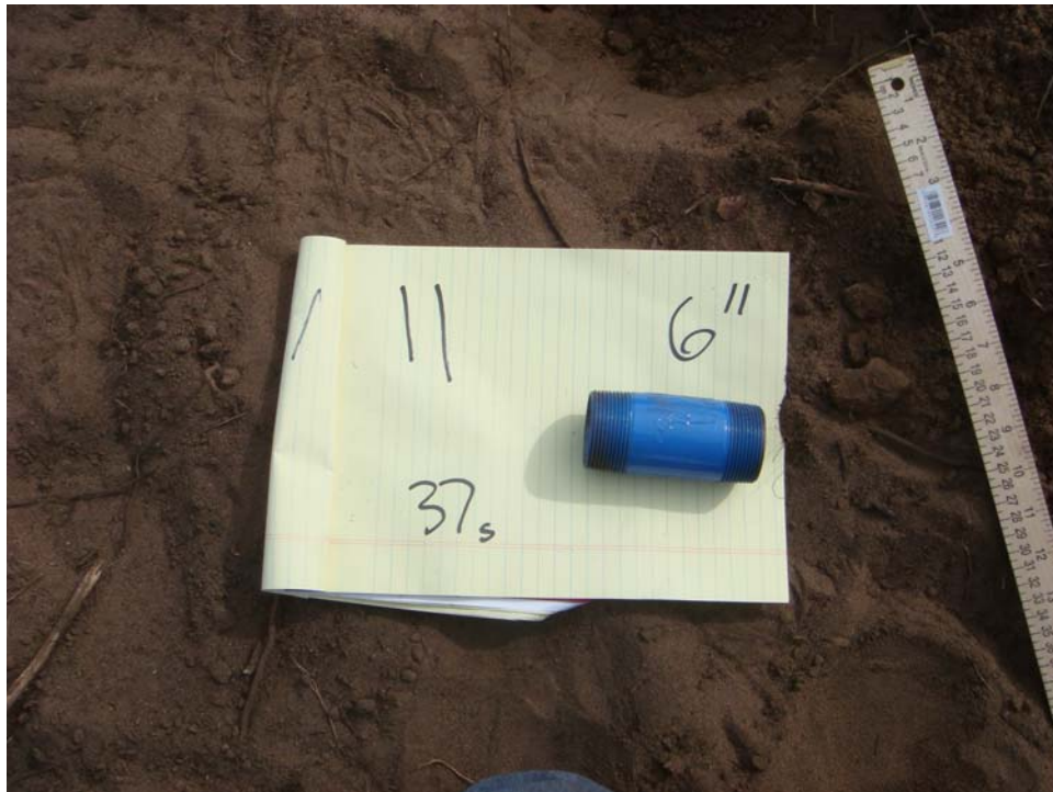
Test Plot 1 - Seed Item 11, 37 mm (pipe short), buried depth = 6 inches
