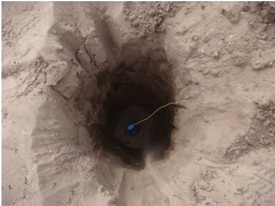
Test Plot 2 - Seed Item 14, Grenade, buried depth = 24 inches
