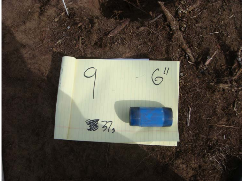
Test Plot 1 - Seed Item 9, 37 mm (pipe short), buried depth = 6 inches
