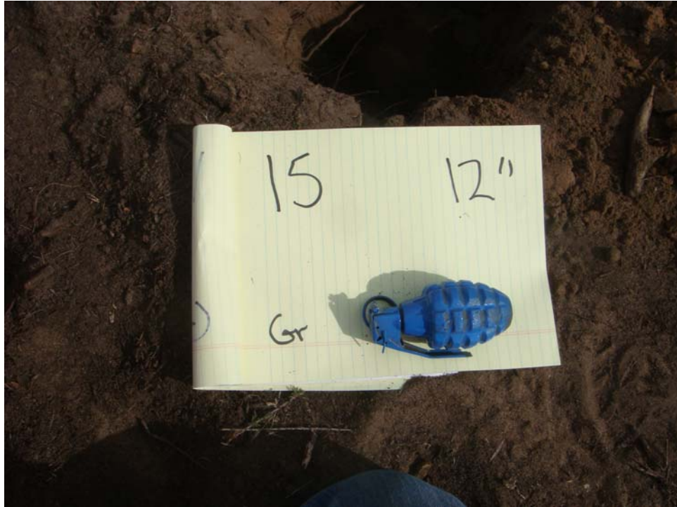
Test Plot 1 - Seed Item 15, Grenade, buried depth = 12 inches
