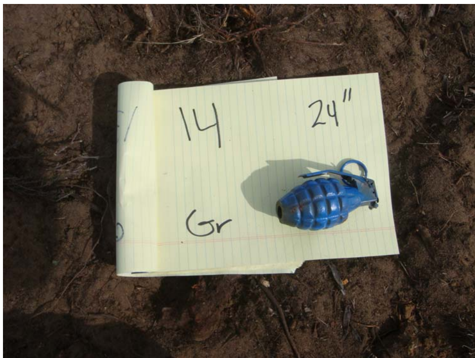
Test Plot 1 - Seed Item 14, Grenade, buried depth = 24 inches
