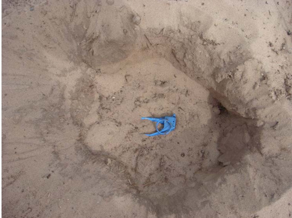
Test Plot 2 - Seed Item 17, Grenade Fuze Assembly, buried depth = 3 inches
