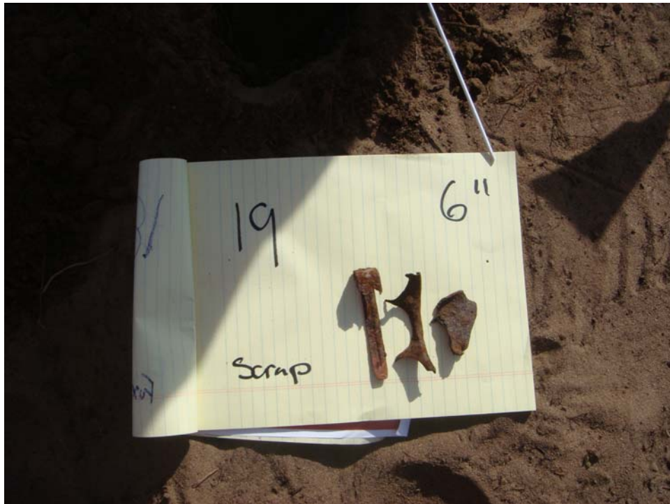
Test Plot 1 - Seed Item 19, Steel Scrap, buried depth = 6 inches
