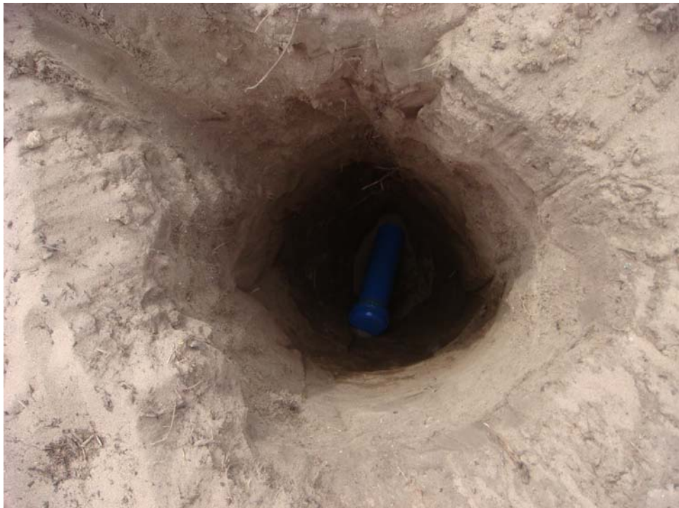
Test Plot 2 - Seed Item 12, 70 mm (pipe), buried depth = 36 inches
