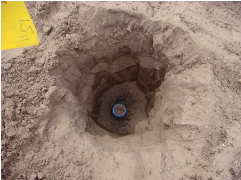
Test Plot 2 - Seed Item 4, 57 mm, buried depth = 12 inches
