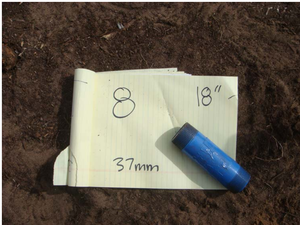
Test Plot 1 - Seed Item 8, 37 mm (pipe), buried depth = 18 inches
