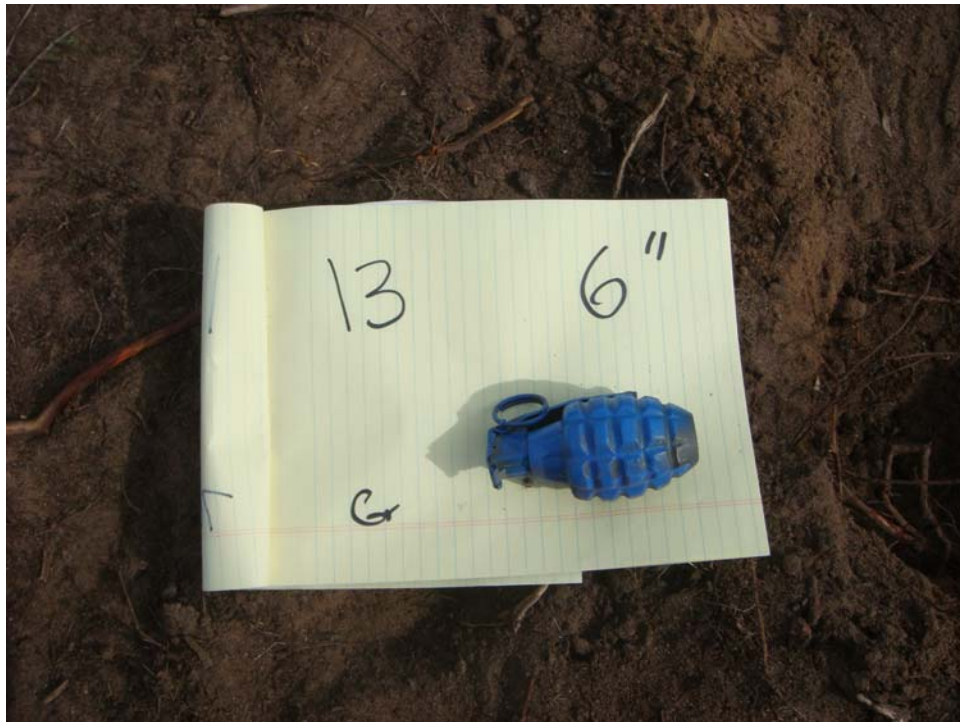
Test Plot 1 - Seed Item 13, Grenade, buried depth = 6 inches
