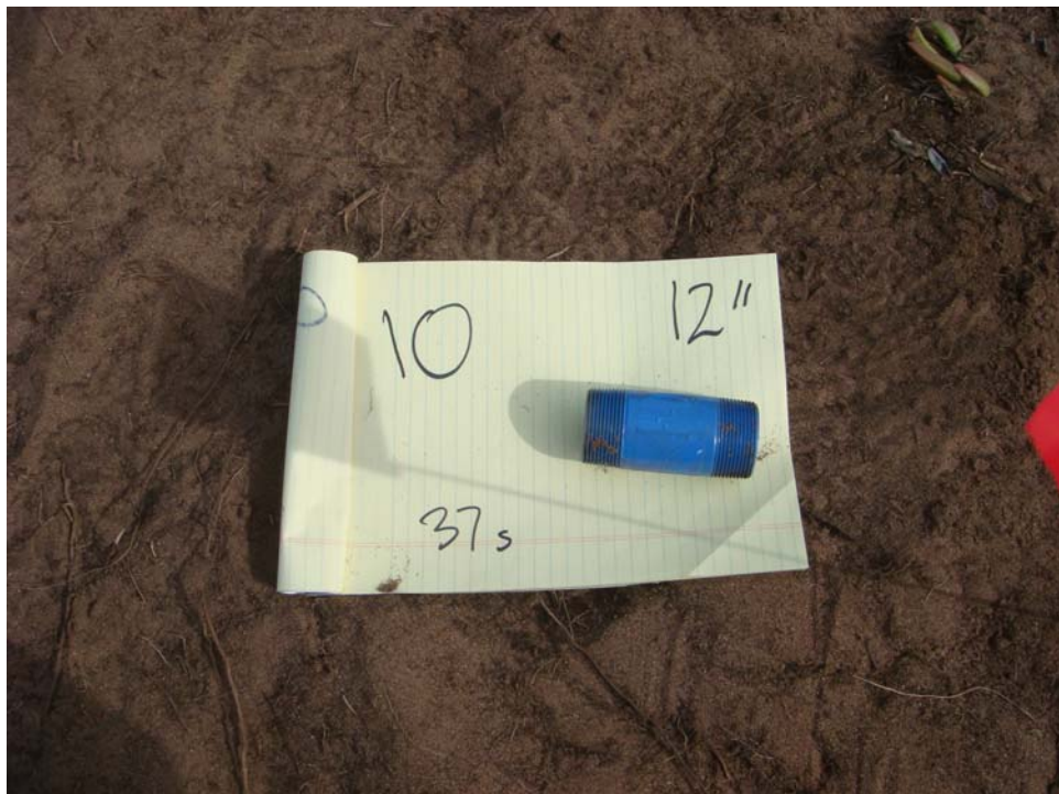
Test Plot 1 - Seed Item 10, 37 mm (pipe short), buried depth = 12 inches
