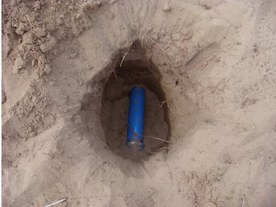
Test Plot 2 - Seed Item 1, 70 mm (pipe), buried depth = 12 inches
