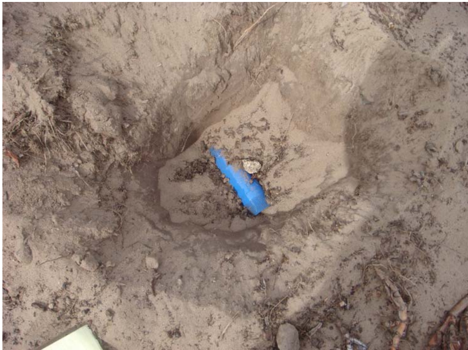
Test Plot 2 - Seed Item 6, 37 mm (pipe), buried depth = 6 inches
