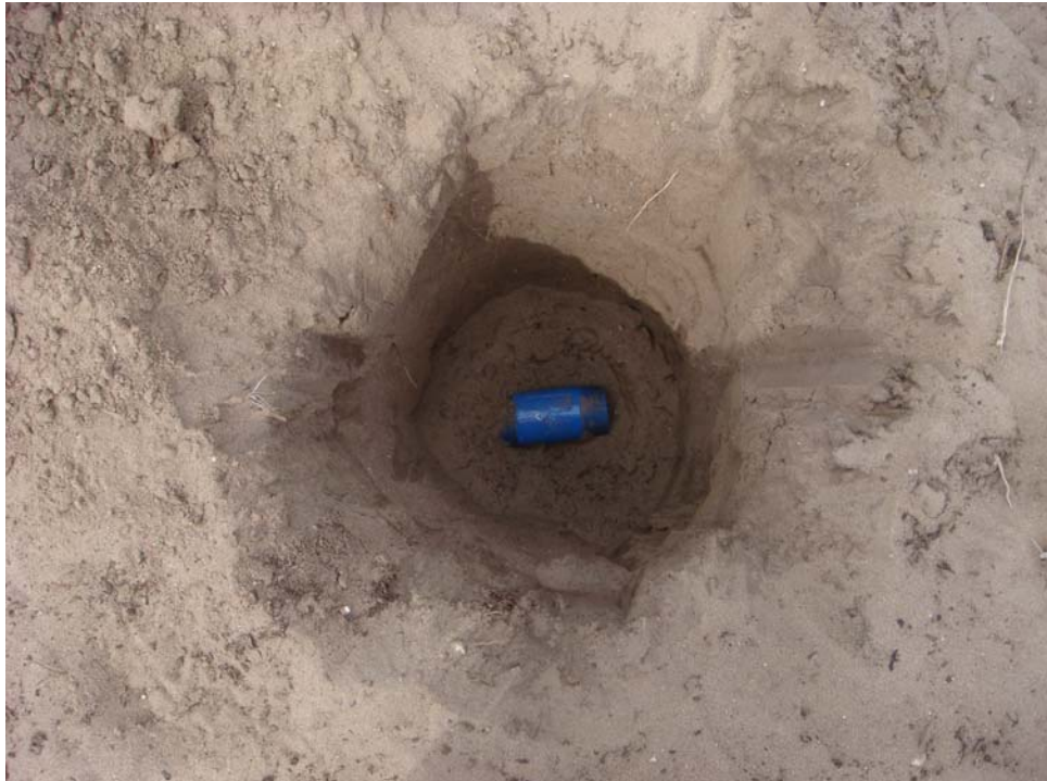
Test Plot 2 - Seed Item 10, 37 mm (pipe short), buried depth = 12 inches
