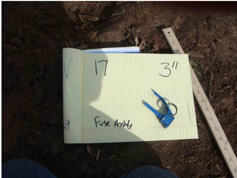
Test Plot 1 - Seed Item 17, Grenade Fuze Assembly, buried depth = 3 inches
