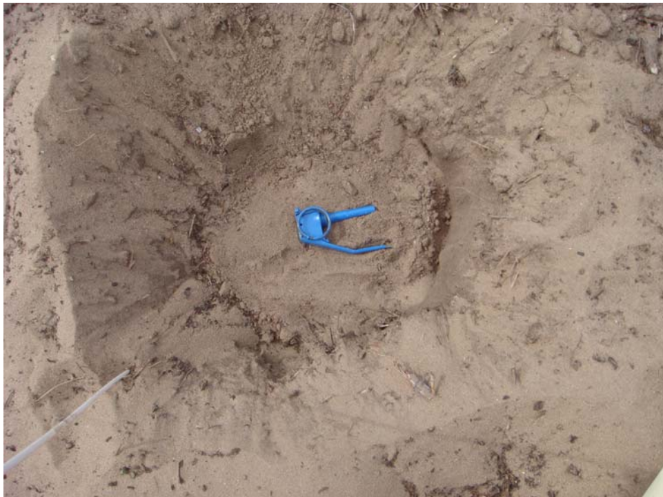
Test Plot 2 - Seed Item 18, Grenade Fuze Assembly, buried depth = 1 inch
