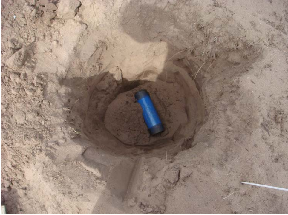
Test Plot 2 - Seed Item 7, 37 mm (pipe), buried depth = 12 inches
