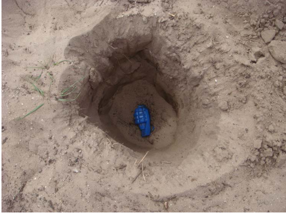
Test Plot 2 - Seed Item 15, Grenade, buried depth = 12 inches
