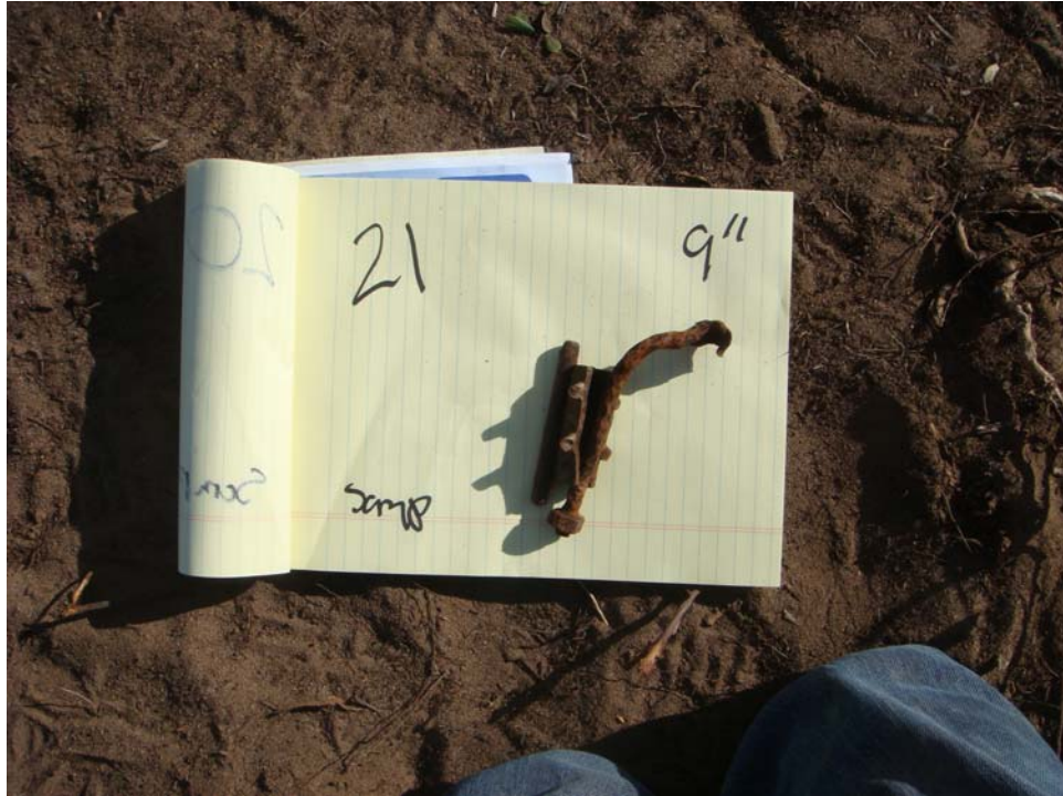
Test Plot 1 - Seed Item 21, Steel Scrap, buried depth = 9 inches
