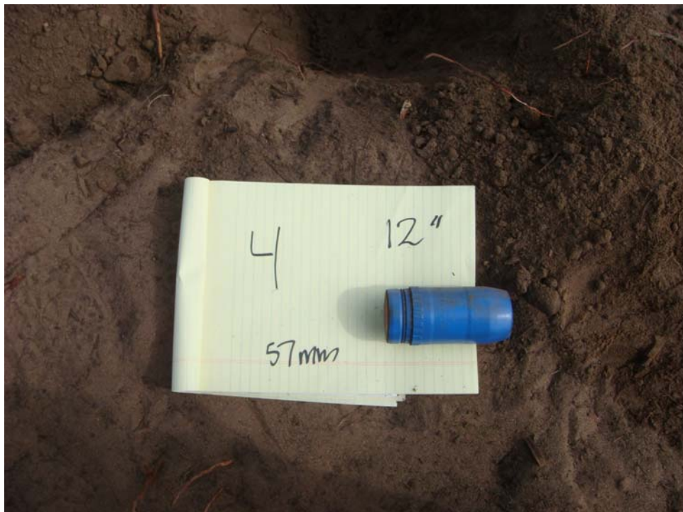
Test Plot 1 - Seed Item 4, 57 mm, buried depth = 12 inches
