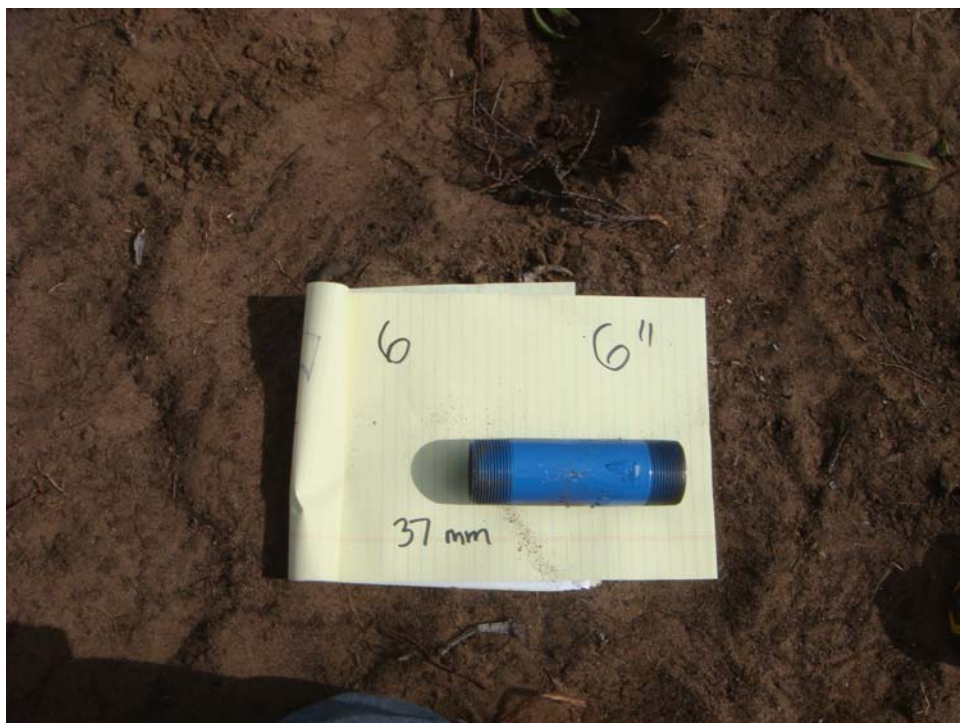
Test Plot 1 - Seed Item 6, 37 mm (pipe), buried depth = 6 inches
