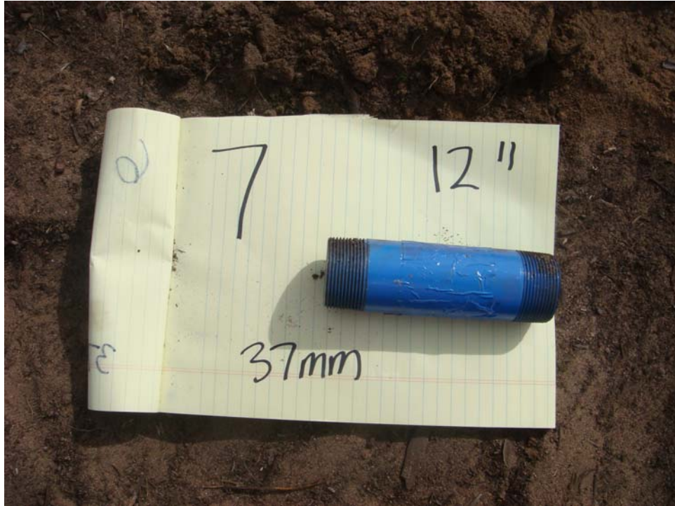
Test Plot 1 - Seed Item 7, 37 mm (pipe), buried depth = 12 inches
