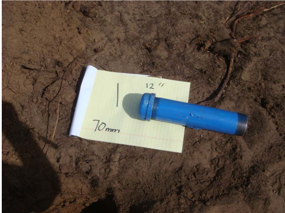
Test Plot 1 - Seed Item 1, 70 mm (pipe), buried depth = 12 inches
