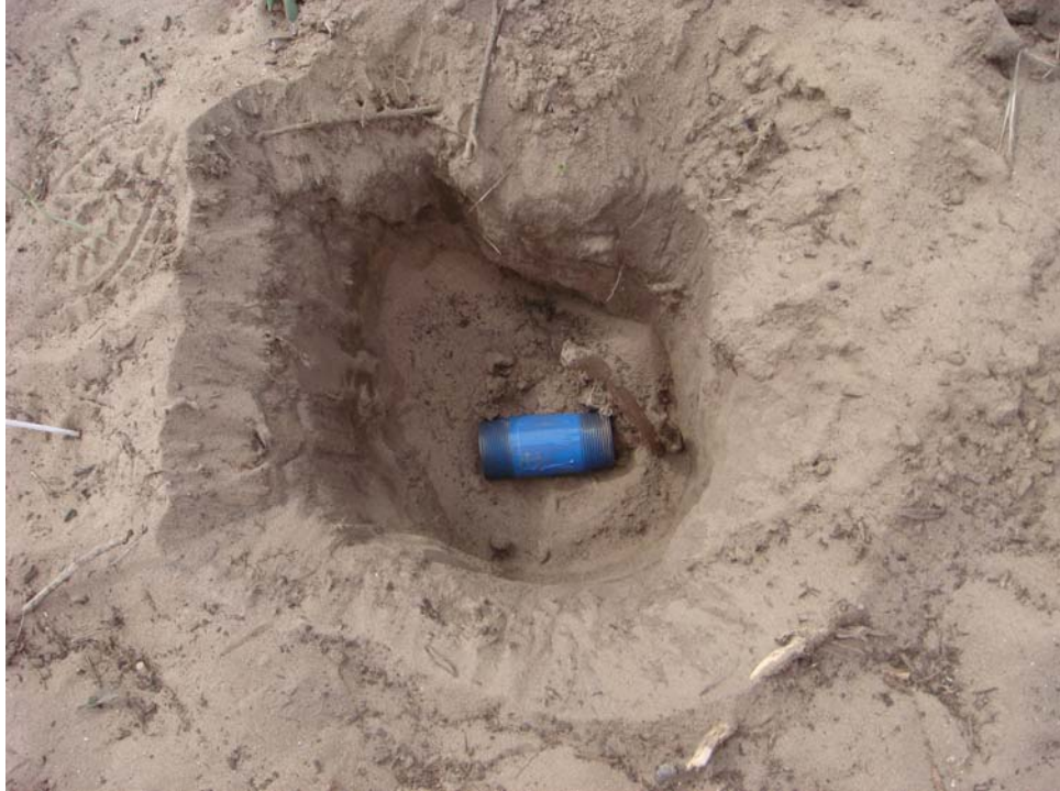
Test Plot 2 - Seed Item 11, 37 mm (pipe short), buried depth = 6 inches
