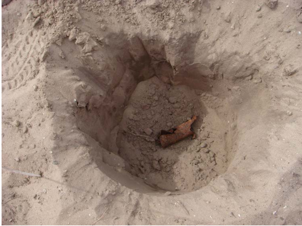
Test Plot 2 - Seed Item 21, Steel Scrap, buried depth = 9 inches
