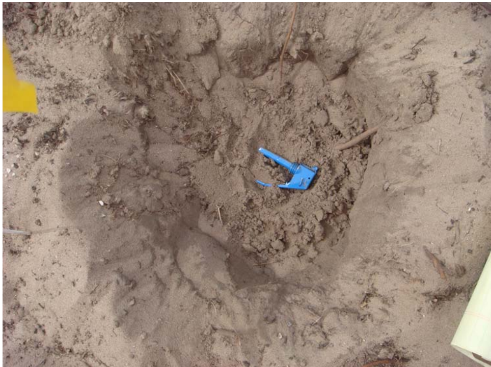
Test Plot 2 - Seed Item 16, Grenade Fuze Assembly, buried depth = 3 inches
