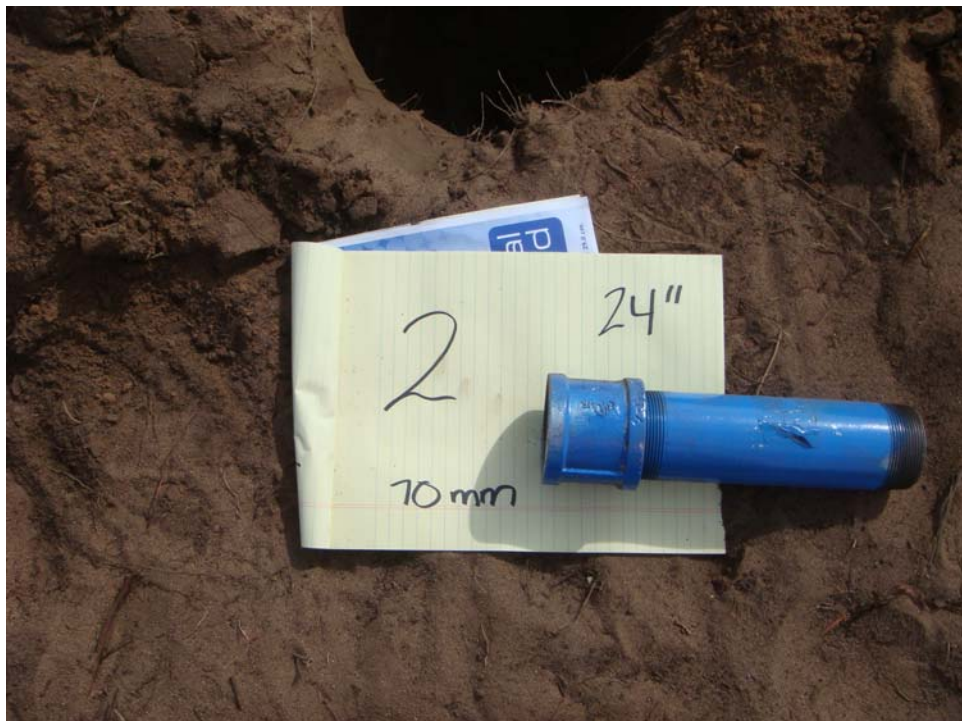
Test Plot 1 - Seed Item 2, 70 mm (pipe), buried depth = 24 inches
