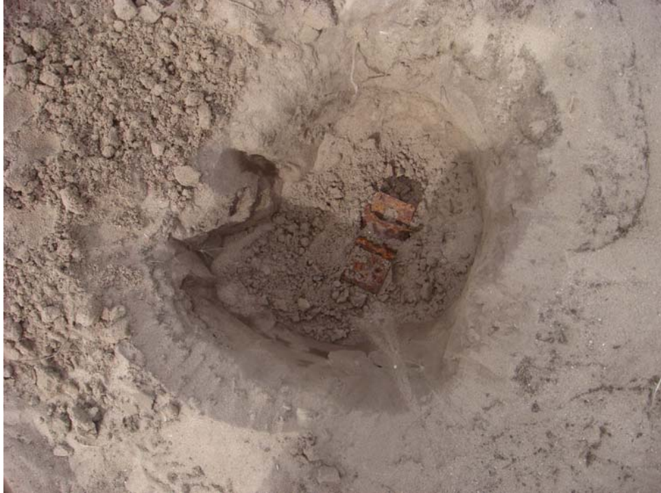
Test Plot 2 - Seed Item 19, Steel Scrap, buried depth = 6 inches
