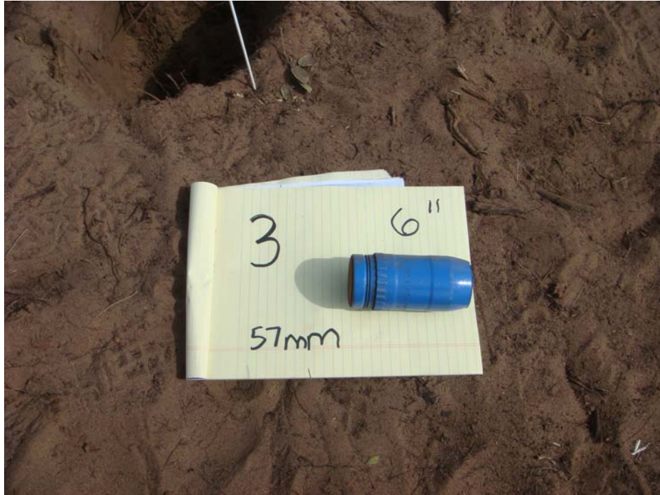
Test Plot 1 - Seed Item 3, 57 mm, buried depth = 6 inches
