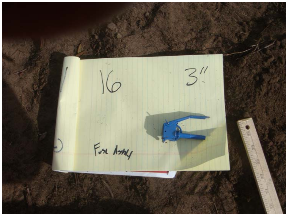
Test Plot 1 - Seed Item 16, Grenade Fuze Assembly, buried depth = 3 inches
