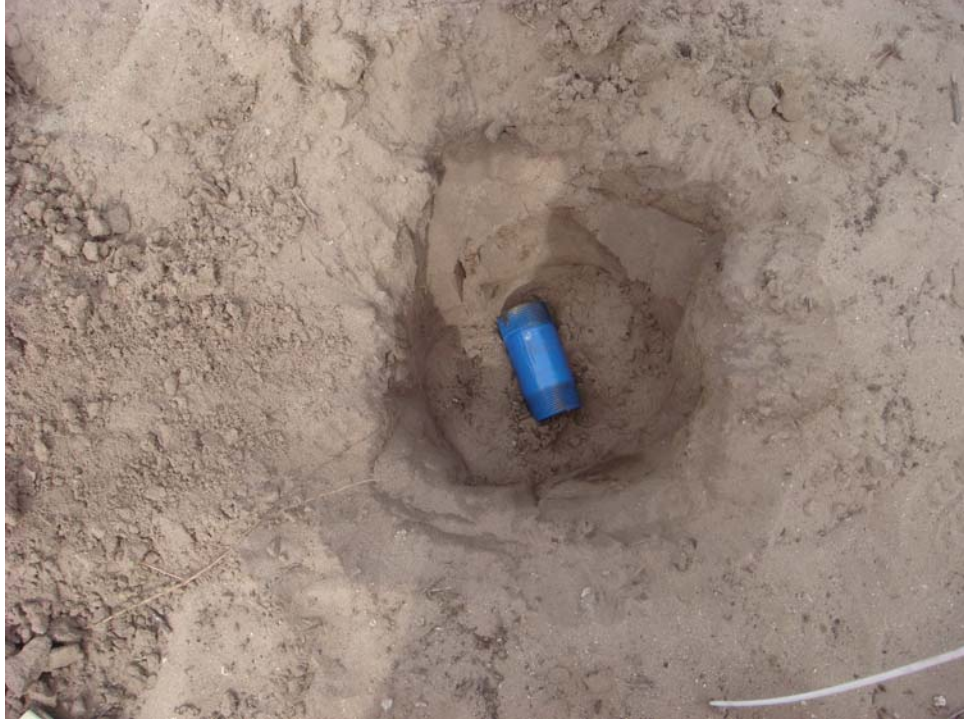
Test Plot 2 - Seed Item 9, 37 mm (pipe short), buried depth = 6 inches
