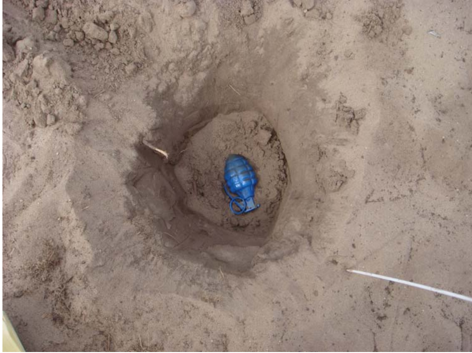
Test Plot 2 - Seed Item 13, Grenade, buried depth = 6 inches
