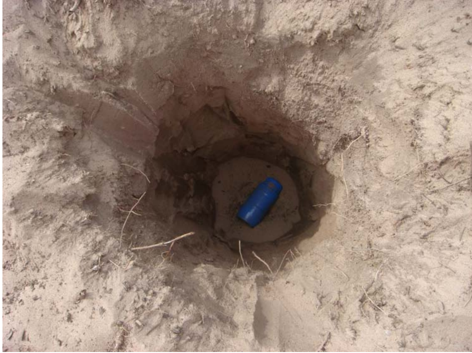
Test Plot 2 - Seed Item 5, 57 mm, buried depth = 24 inches
