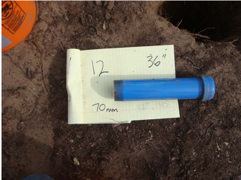
Test Plot 1 - Seed Item 12, 70 mm (pipe), buried depth = 36 inches
