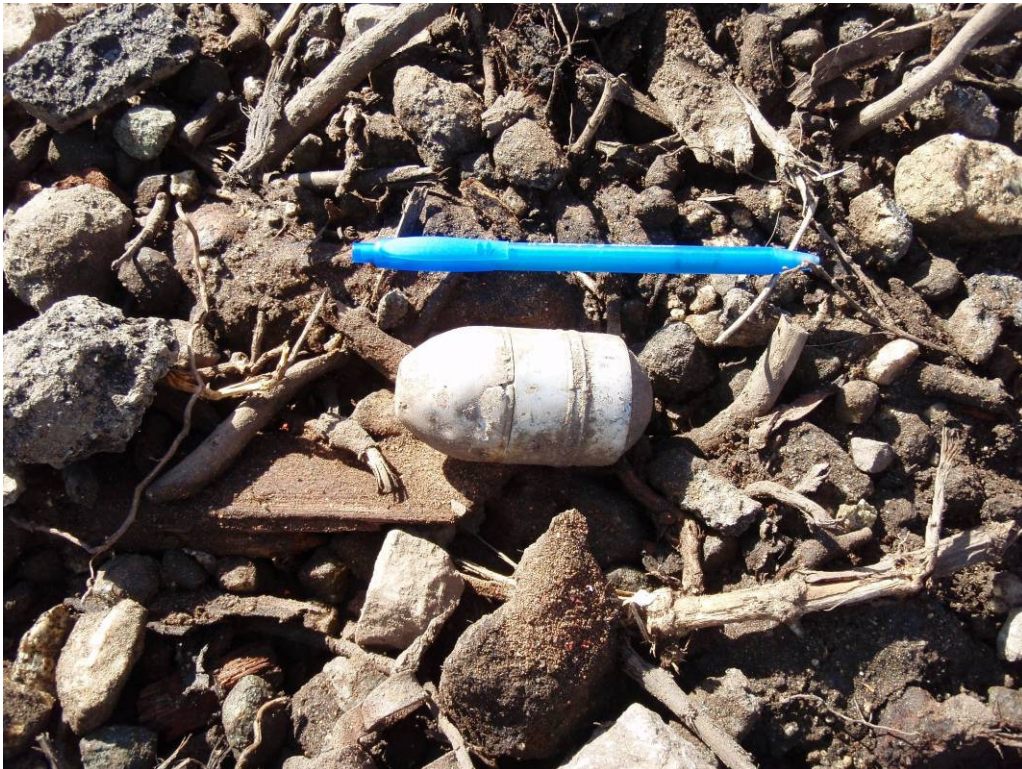
Photograph 16: June 18, 2008. M407A1, 40mm, practice. Recovered during soil sifting activities for soil from MRS-15SEA.4.
