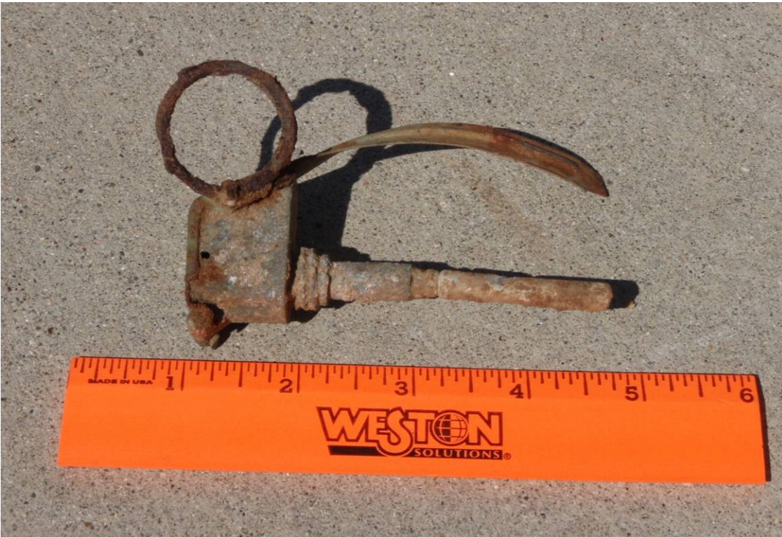
Photograph 18: June 26, 2008. Hand grenade fuze. Recovered during DGM anomaly investigation in hillside west of GJMB.
