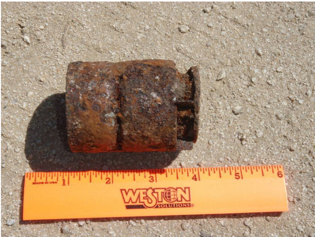
Photograph 10: June 10, 2008. Fuze, mine, antitank, practice, M1A1 (safety clip in place). Recovered during soil sifting activities for soil from MRS-15SEA.4.
