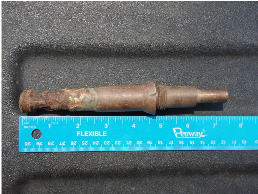
Photograph 11: June 12, 2008. Fuze, PD, French No. 5. Recovered during soil sifting activities for soil from MRS-15SEA.4.
