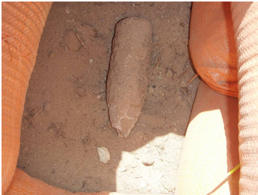
Photograph 20: July 22, 2008. Projectile, 57mm, HE M306. Recovered during DGM anomaly investigation in SCA_W140 on MRS-15SEA.4.
