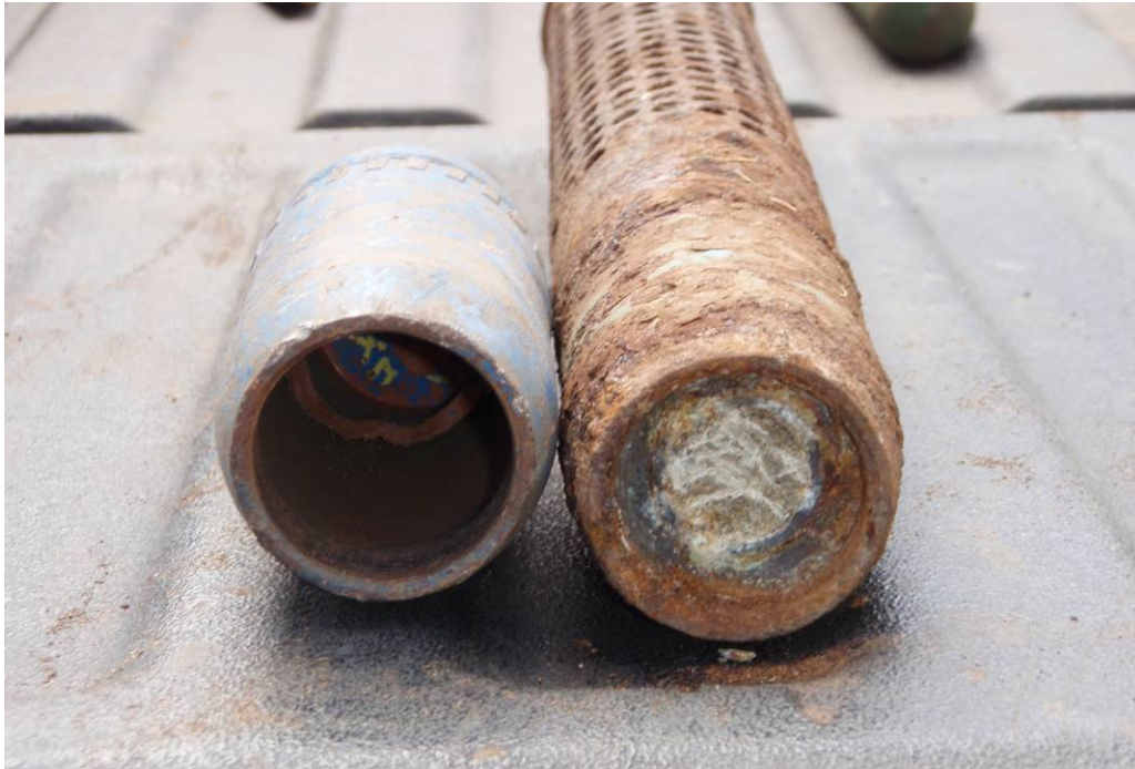
Photograph 9: June 4, 2008. Cartridge, 57mm, TP M306A1 (includes projectile, unfuzed). Recovered during soil sifting activities for soil from MRS-15SEA.4.
