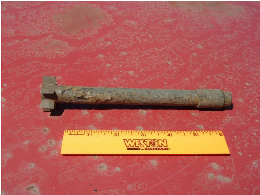
Photograph 19: July 15, 2008. Rocket, 35mm, subcaliber, practice, M73. Recovered during soil sifting activities for soil from MRS-15SEA.4.
