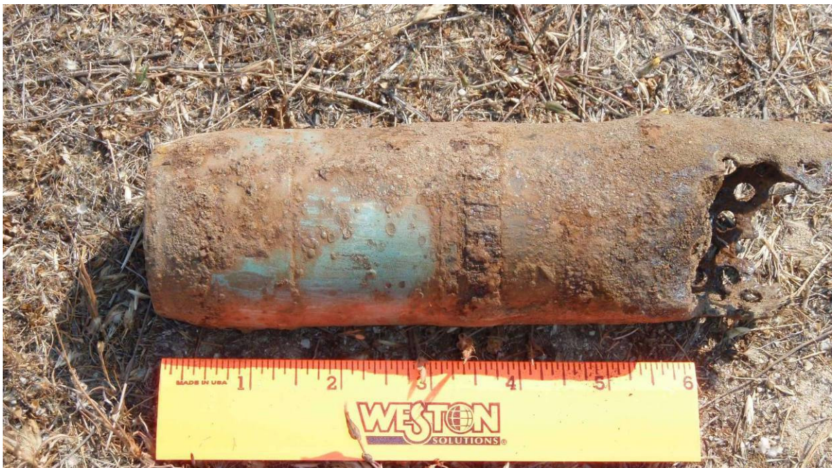
Photograph 12: June 12, 2008. Projectile, 57mm, TP M306 (unfuzed, unfired with possible spotting charge). Recovered during soil sifting activities for soil from MRS-15SEA.4.
