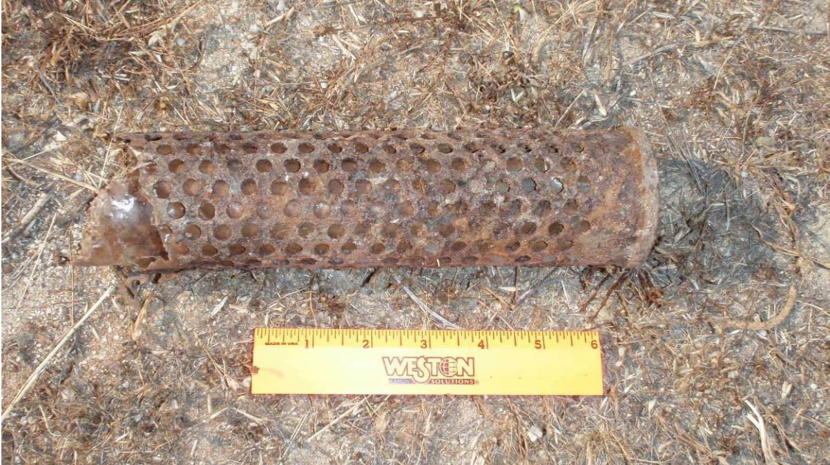
Photograph 15: June 17, 2008. Cartridge, 57mm, M60A1 (no projectile, primer live). Recovered during soil sifting activities for soil from MRS-15SEA.4.
