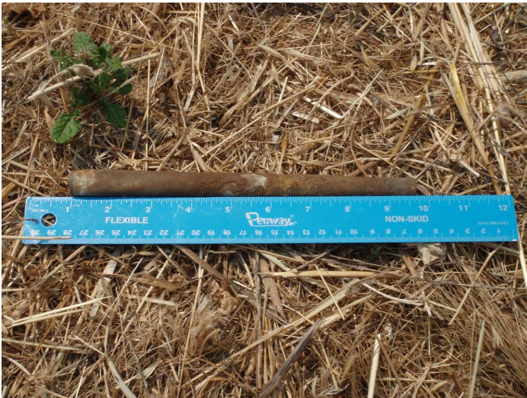
Photograph 14: June 13, 2008. Burster tube. Recovered during DGM anomaly investigation in SCA_W048 on MRS-15SEA.1.
