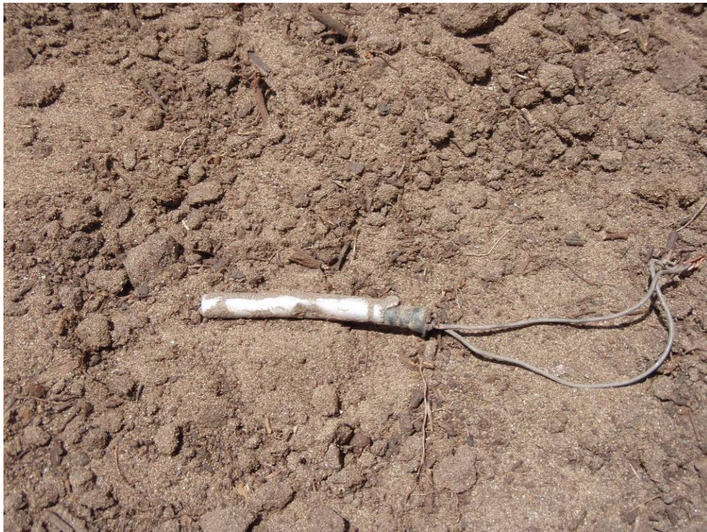
Photograph 7: May 28, 2008. Cap, blasting, electrical, M6. Recovered during soil sifting activities for soil from MRS-15SEA.1.
