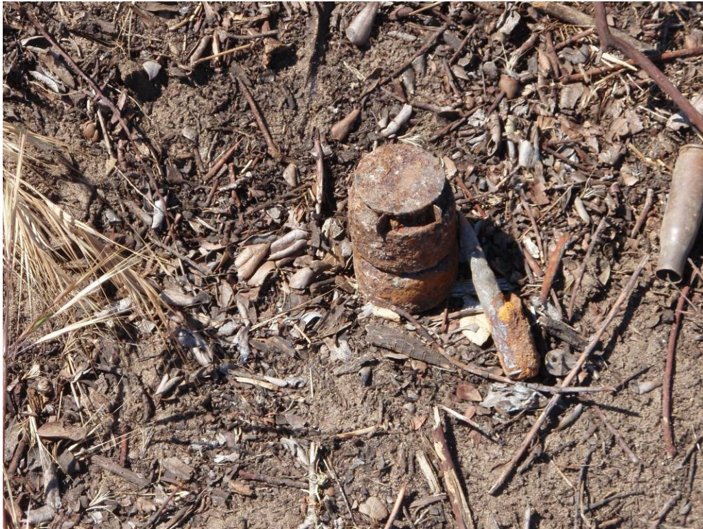
Photograph 13: June 13, 2008. Fuze, mine, antitank, practice, M1A1 (safety clip in place). Recovered during soil sifting activities for soil from MRS-15SEA.4.
