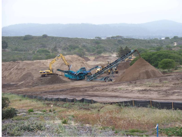
Photograph 3-14 – Sifting plant operations
