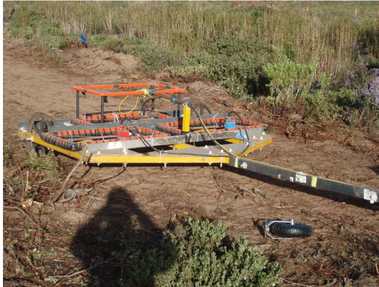
Photograph 3-2 - EM61-MK2 vehicle-towed multi-array system
