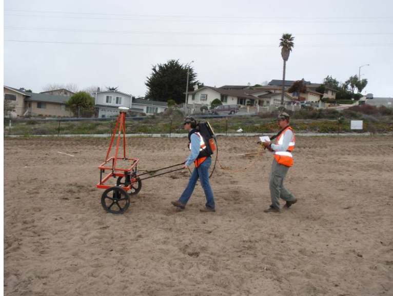
Photograph 3-1 - EM61-MK2 man-towed single-array system
