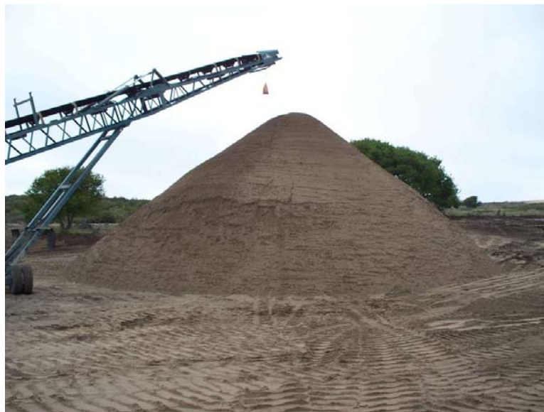
Photograph 3-17 – Final screened material from the sifting plant
