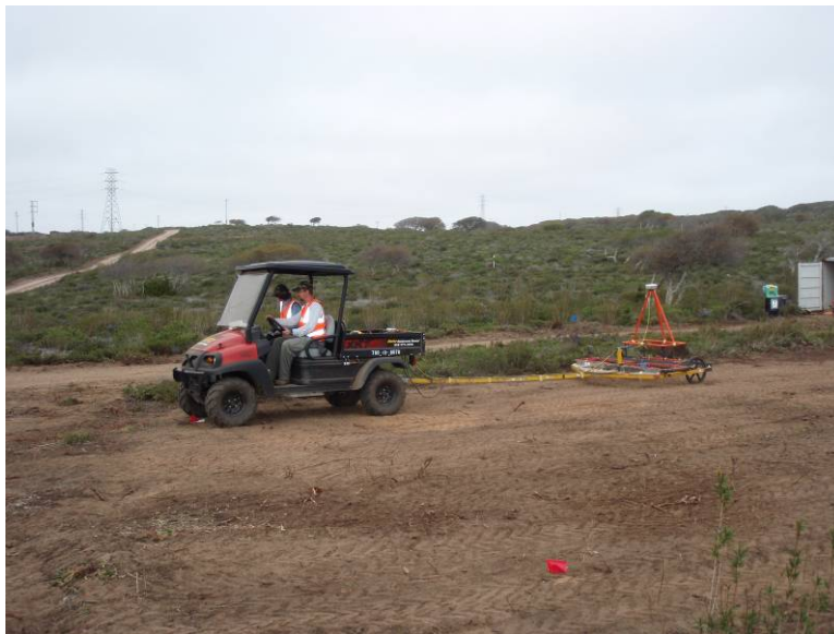
Photograph 3-3 - EM61-MK2 vehicle-towed multi-array system
