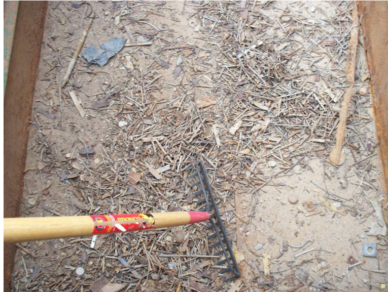
Photograph 3-16 – Metal recovered from the second magnet of the sifting plant
