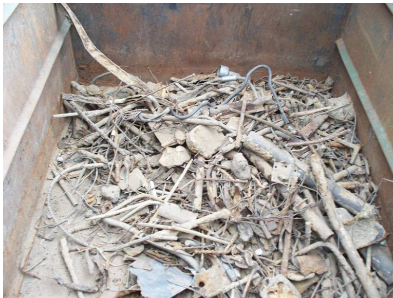
Photograph 3-15 – Metal recovered from the first magnet of the sifting plant
