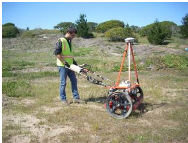
Photo 3-2 – EM61-MK2 Wheeled Cart at 8-Inch Coil Height
