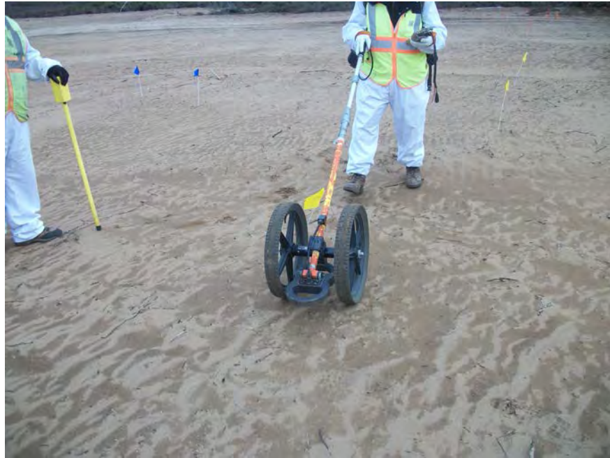
Picture 1: Anomaly locating with the EM 61 IAR Rg 47
