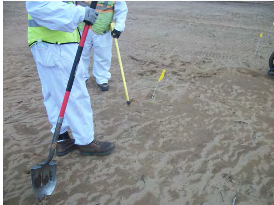
Picture 2: Anomaly pinpointing using a Schonstedt IAR Rg 47
