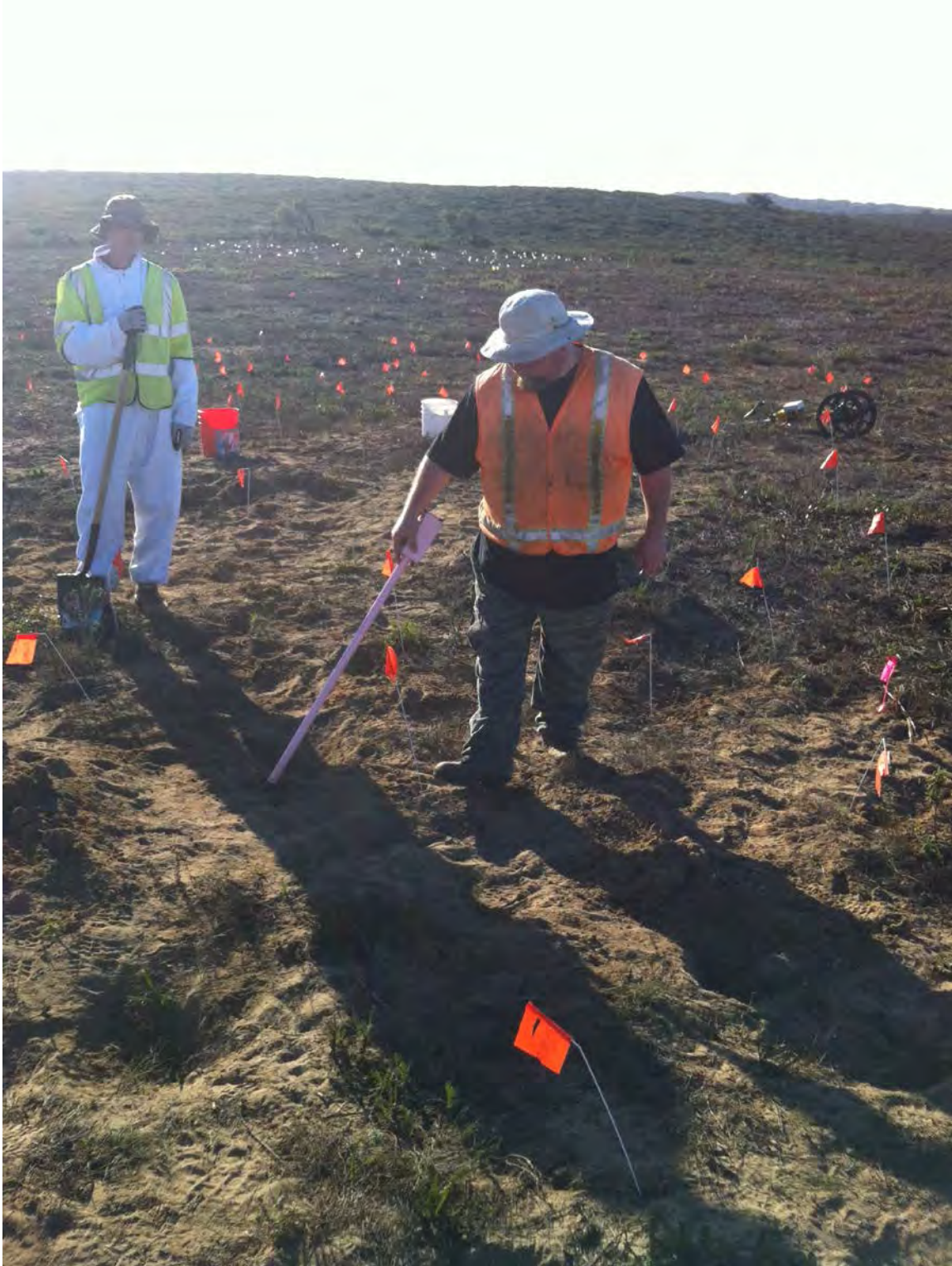
Picture 3: Pinpointing an anomaly utilizing a Shconstedt
