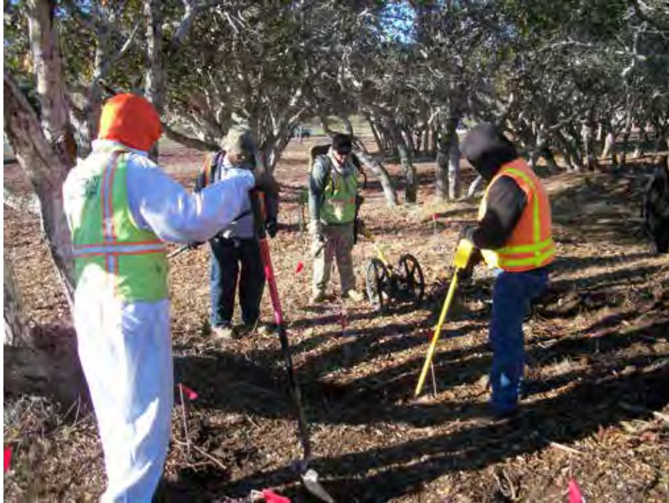
Picture 1: Personnel performing all procedures; anomaly acquisition, pinpointing, and excavation IAR Range 47 SCA
