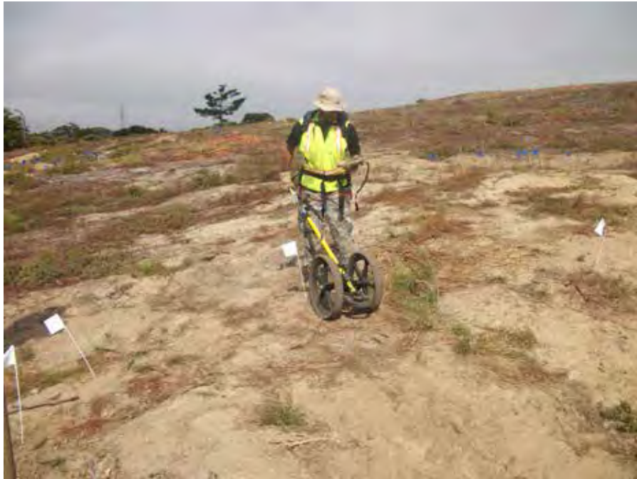
Picture 1: Employment of EM 61 HH for Target Investigation in Grid B1B8F5
