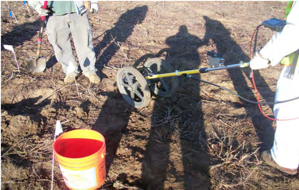
Picture 3: Anomaly locating utilizing the EM61
