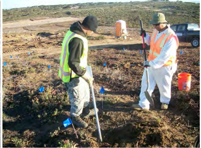
Picture 1&2: Anomaly locating with the EM 61 and pinpointing utilizing Schonstedt IAR R 44 North SCA
