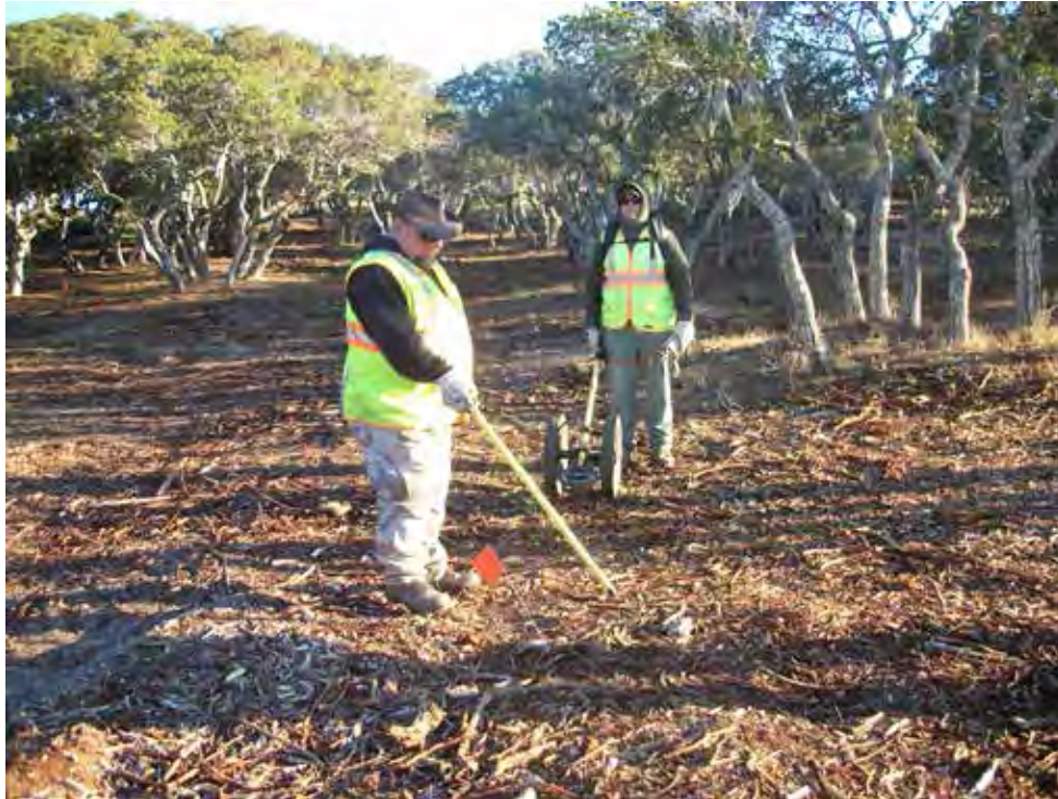
Picture 3: UXO Technician pinpointing with Schonstedt detector IAR Range 47SCA
