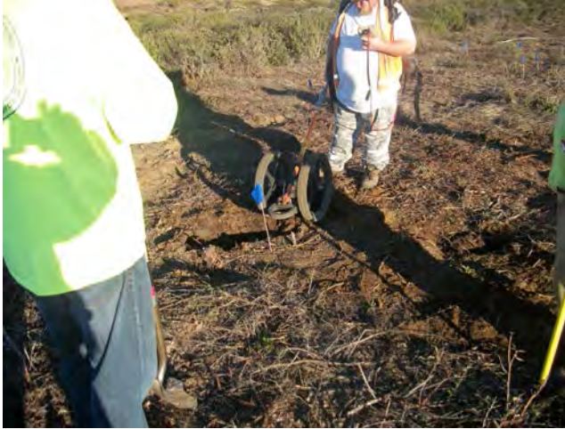
Pics 1&2 anomaly investigations using an EM 61 and a Schonstedt
