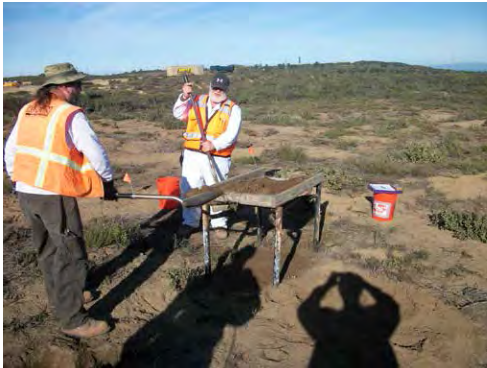
Picture 3: Sift table used on soils with concentrated small anomalies IAR Range 47SCA
