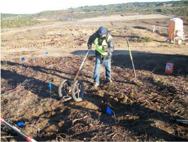
Picture 1&2: Anomaly locating with the EM 61 and pinpointing utilizing Schonstedt IAR R 44 North SCA
