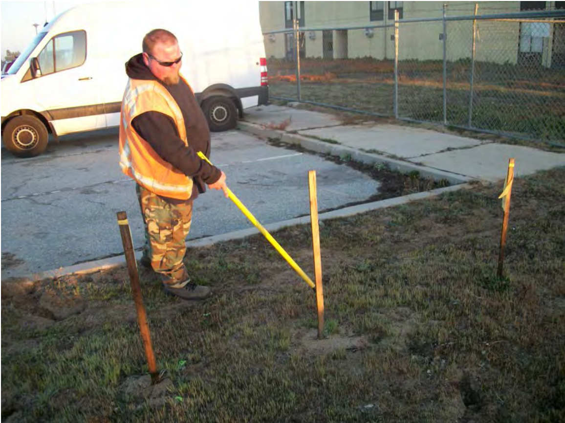
Picture 1: Shconstedt function check prior to operations
