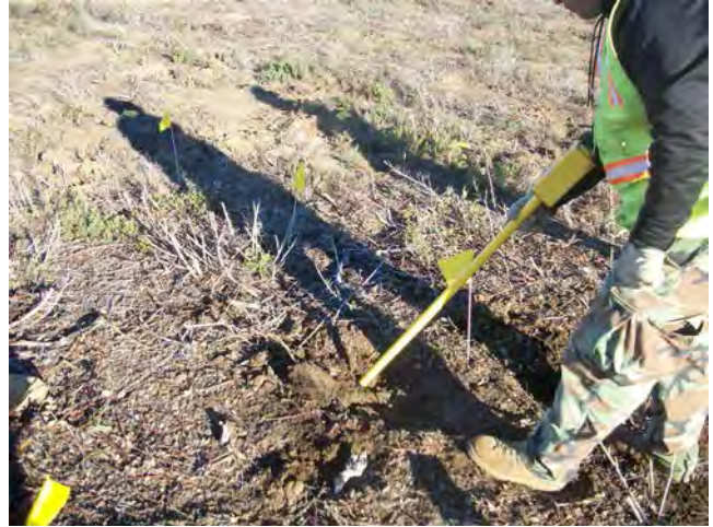
Pics 1&2 anomaly investigations using an EM 61 and a Schonstedt
