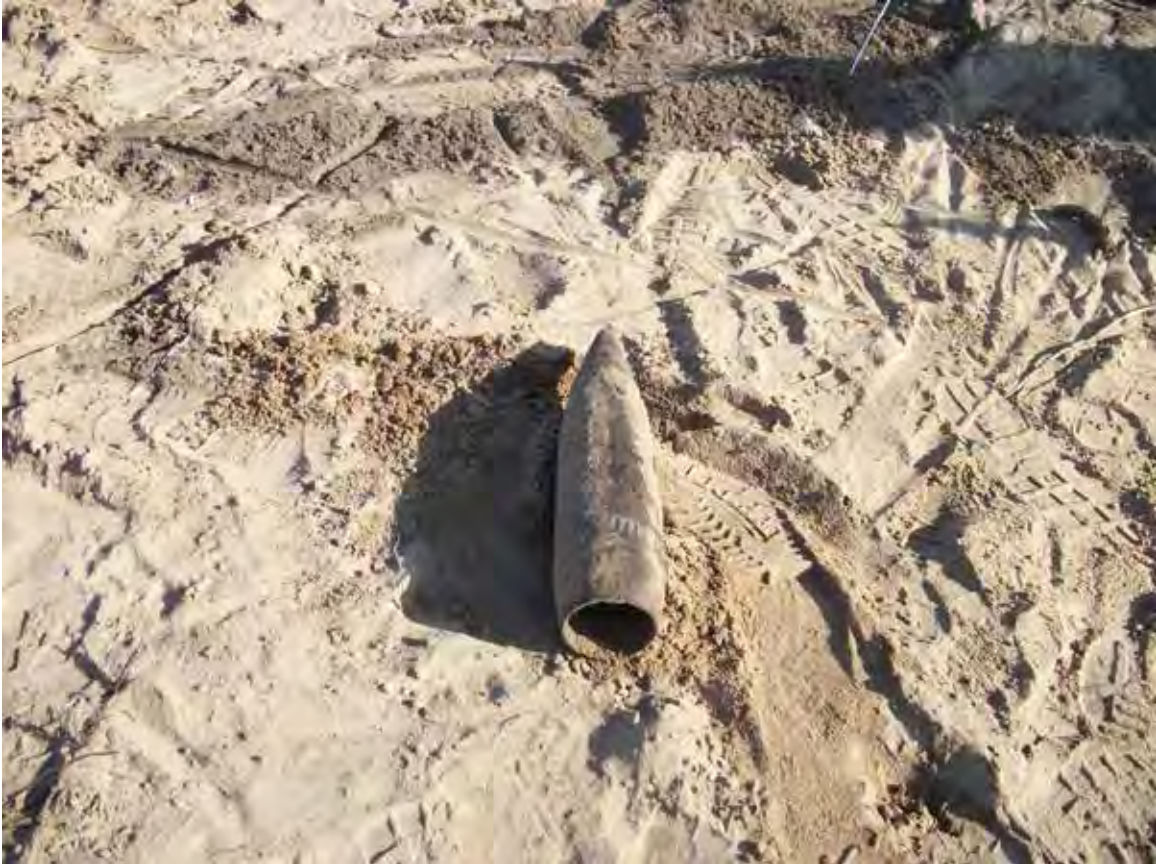
Picture 3: Expended 105MM, M314 projectile
