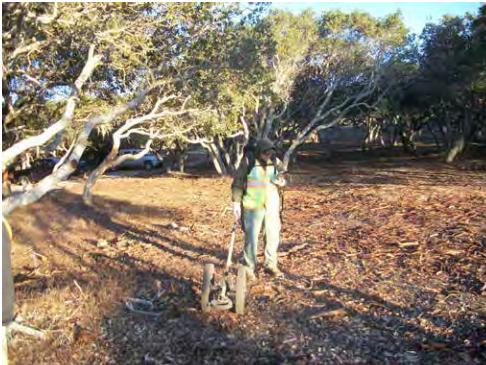
Picture 2: EM 61 utilized for anomaly acquisition IAR Range 47 SCA
