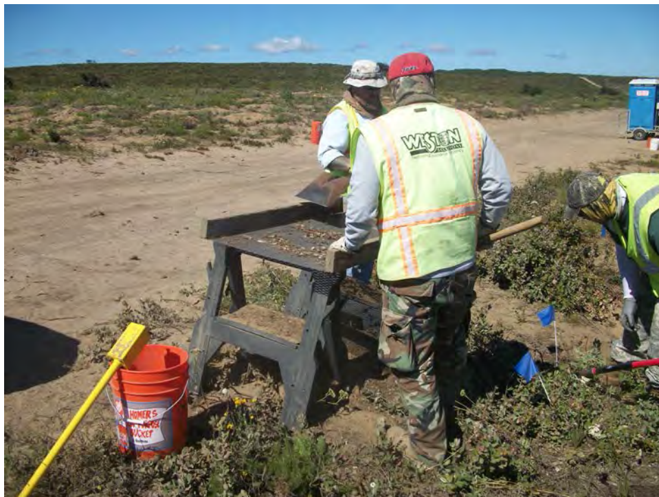
Pic 2: Using a sift table in grid operations IAR MRA
