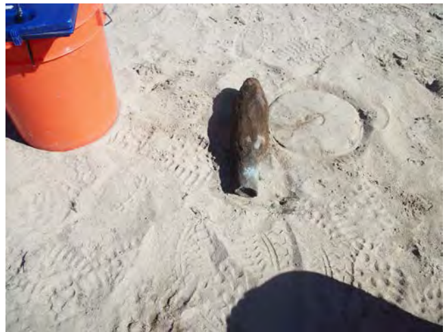
Pic 4: MD, partial M29, 3.5 inch rocket
