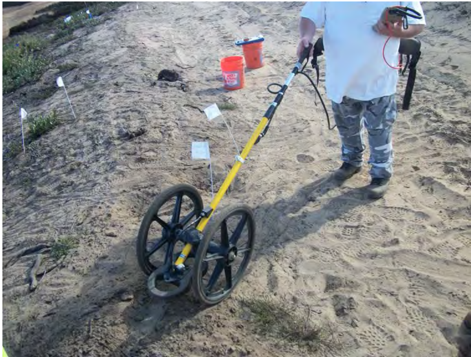
Picture 3: Proper usage of EM61
