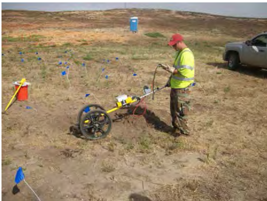
Picture 1: Employment of EM 61 HH for Target Investigation in Grid B1B8F5
