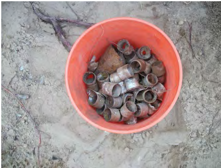
Picture 3: Munitions Debris (40mm M407 components) found during Sifting Operations in the Interim Action Range Range 47 Sifting operations
