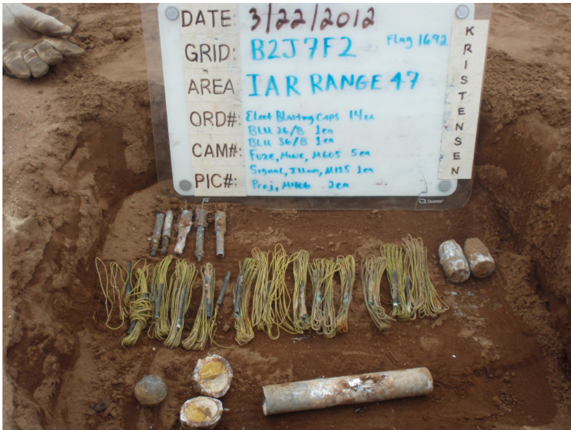
Photograph 2 - Cap, Blasting, Electric, M6; Bomb, BLU-26/B, Training; Bomb, BLU-36/B, Training; Fuze, Mine, Combination, M605; Signal, Illumination, Ground, M125; Projectile, 40mm, High Explosive, M406
