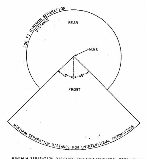
MINIMUM SEPARATION DISTANCE FOR UNINTENTIONAL DETONATIONS USING MINIATURE OPEN FRONT BARRICADE DURING INTRUSIVE ACTIVITIES
