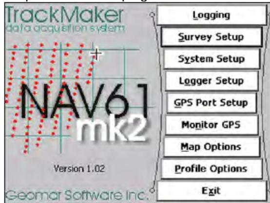
4. Click on “Survey Setup” and specify the below options. For analog operation, the Mode is set to “Auto” and Readings/s is set to “5”.
