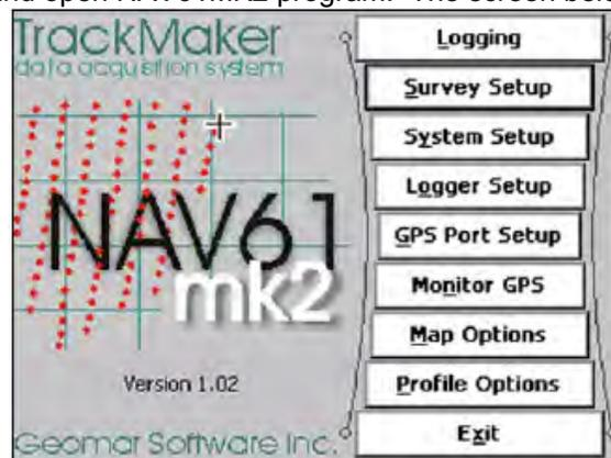
4. Click on “Survey Setup” and specify the below options. For target reacquisition, the Mode is set to “Auto” and Readings/s is set to “5”.
