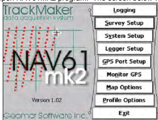
4. Click on "Survey Setup" and specify the below options. For this GPS/RTK Method, the Mode is set to "Auto" and Readings/s is set to "10".
