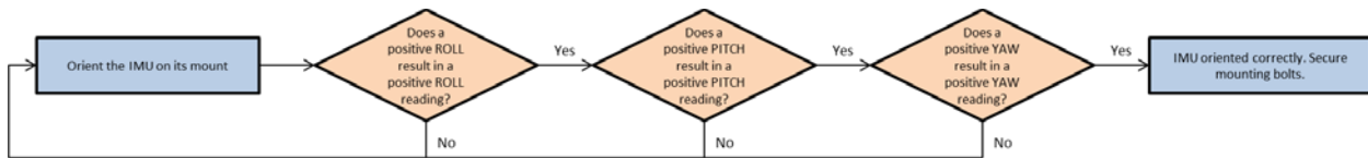
Figure 4. Procedure for verification of IMU orientation
