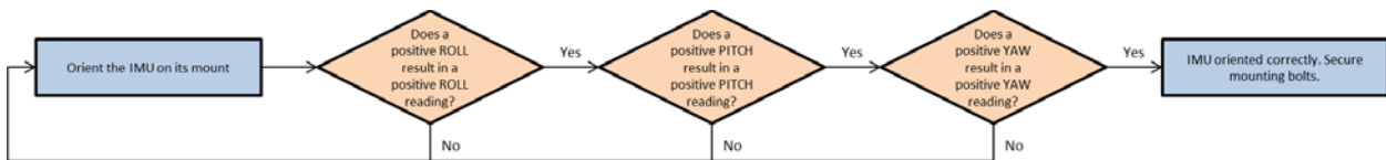
Figure 12. Procedure for verification of IMU orientation
