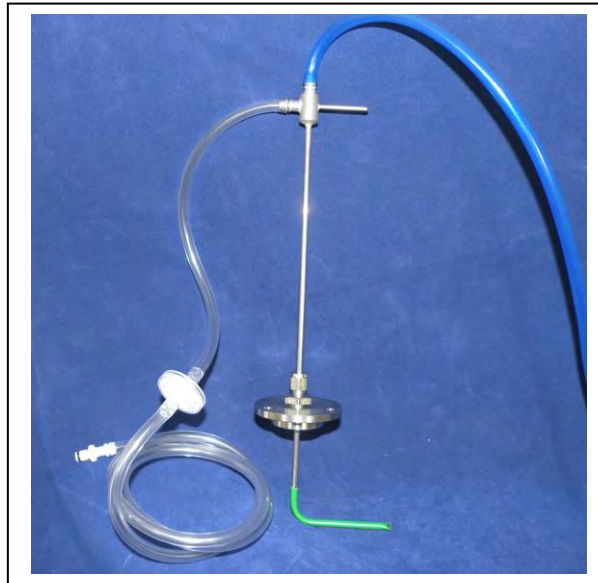
Example of a pitot tube
