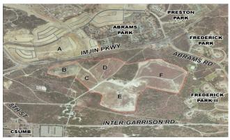
As part of the Superfund cleanup, the Army has installed a groundwater extraction and treatment facility, which has been operating since 1995. To prevent further migration of contaminants into the groundwater, an engineered cover system has been installed over areas B through E in three phases (1997-2013).
